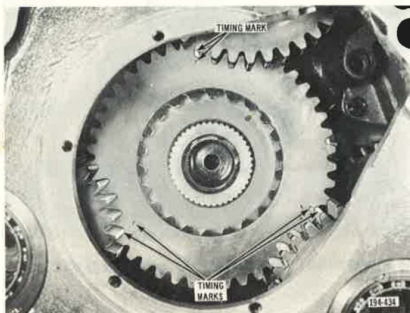
Figure 62. Aligning "O" Marks on Lo-Range Gear with Countershaft Gears
