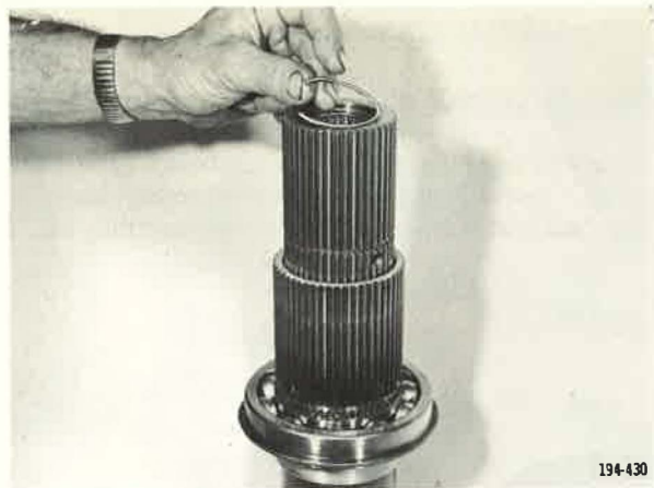
Figure 29. Removing Roller Bearing Retaining Snap Ring
