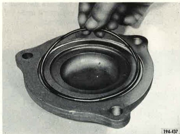
Figure 66. Installing Rear Countershaft Rear Bearing Cover O-Ring
