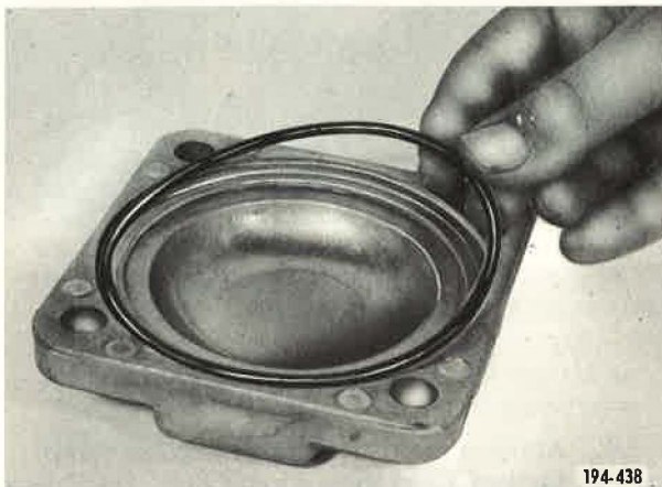
Figure 42. Installing Front Countershaft Front Bearing Cover O-Ring
