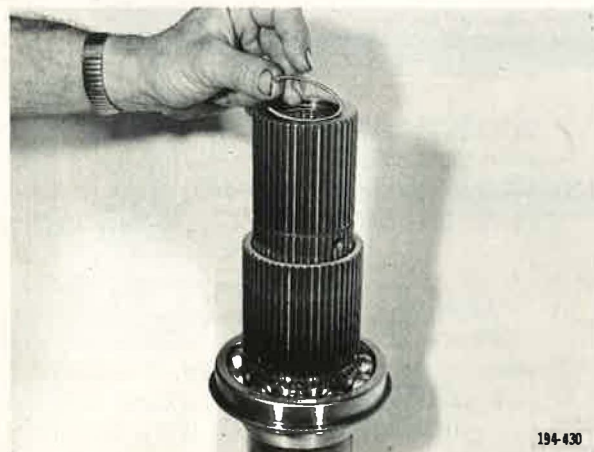
Figure 33. Installing Front Roller Bearing Snap Ring
