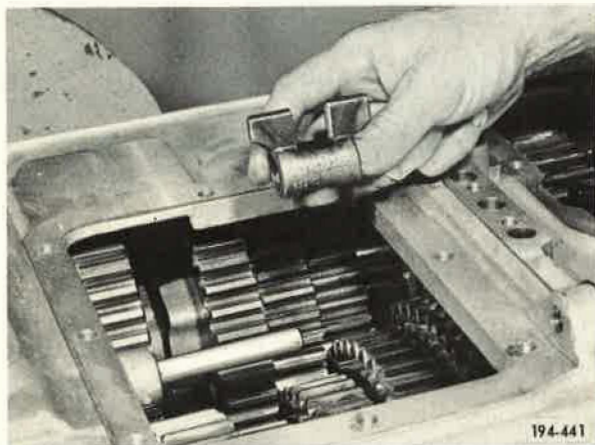
Figure 69. Installing Second and Third Speed Shifter
