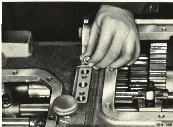
Figure 72. Installing Shift Rail Poppet Ball
