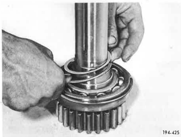
Figure 25. Removing Pinion Bearing Retaining Spirollox Snap Ring
