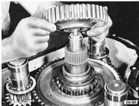
Figure 6. Removing Lo-Range Main Drive Gear
