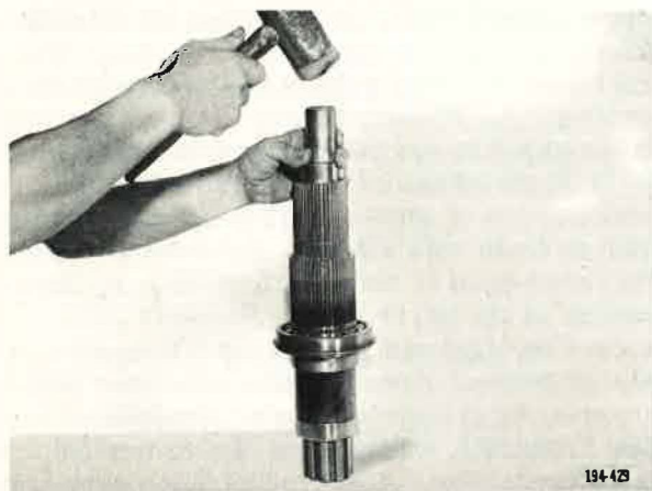
Figure 32. Installing Front Roller Bearing
