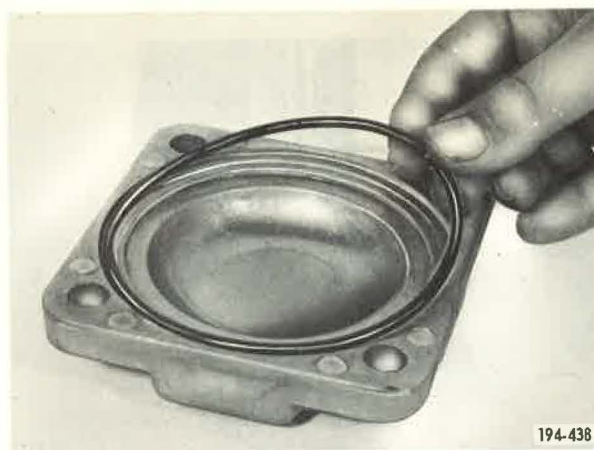
Figure 21. Installing Bearing Cover O - Ring
