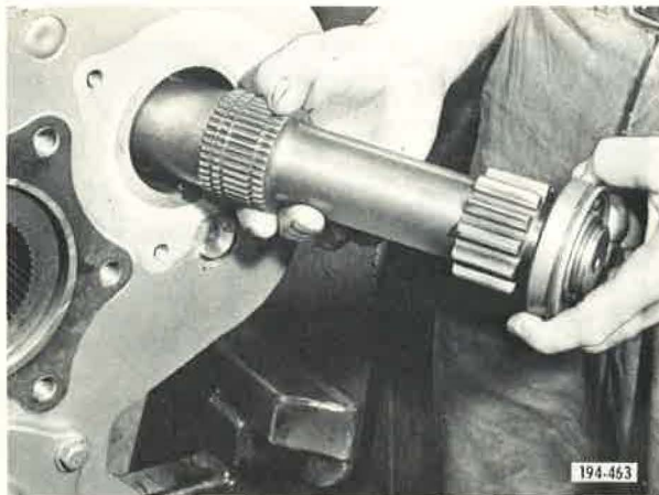
Figure 30. Installing Rear Countershaft
