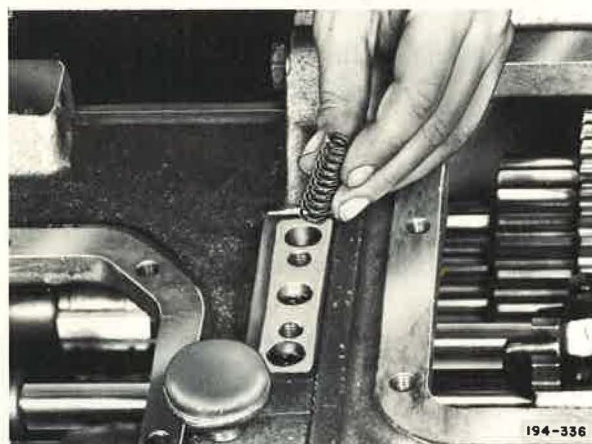
Figure 47. Installing Shift Rail Poppet Ball
