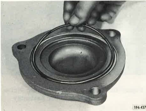
Figure 33. Installing O-Rings in Rear Bearing Cover
