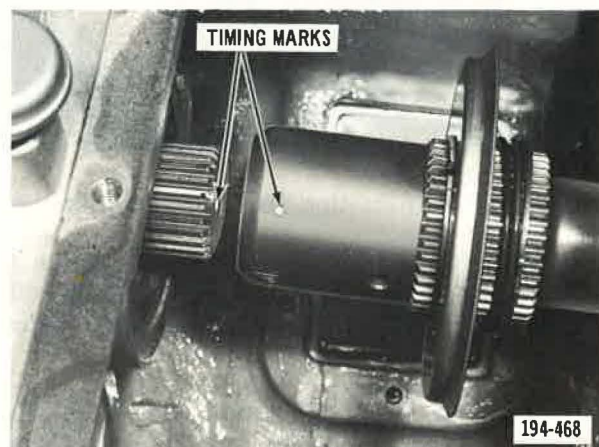
Figure 32. Aligning Timing "O" Mark on Rear Countershaft with Front Countershaft
