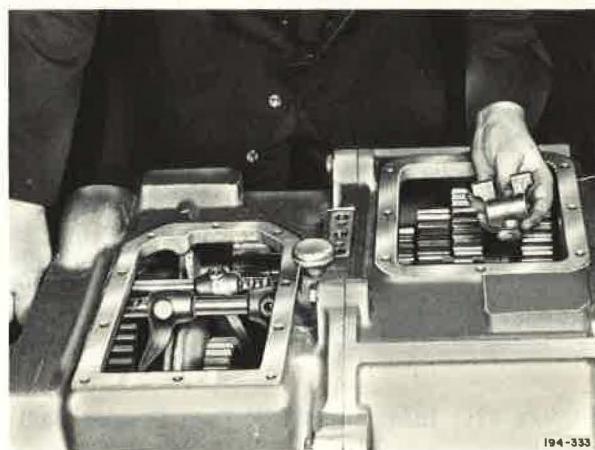
Figure 45. Installing Second and Third Speed Shifter
