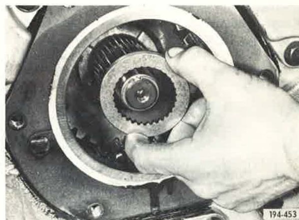
Figure 7. Removing Fourth Speed Gear Selective Thrust Washer
