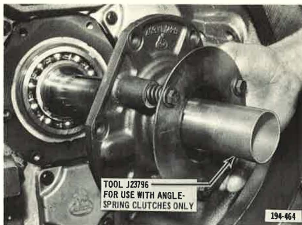
Figure 40. Installing Main Driving Pinion Bearing Cover Assembly
