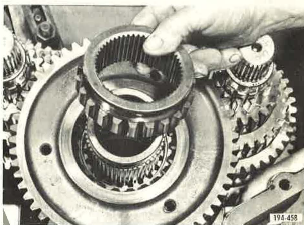
Figure 27. Installing First Speed Sliding Clutch
