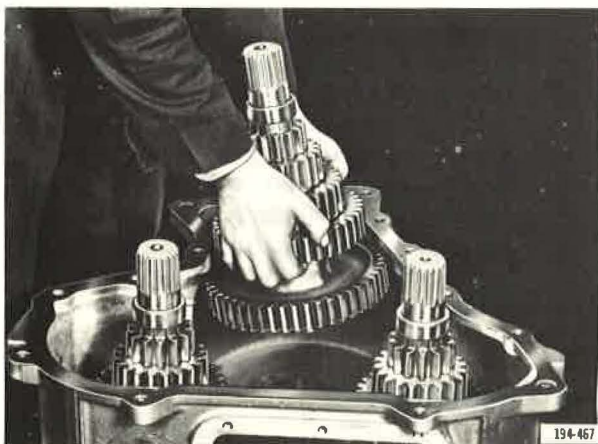
Figure 15. Removing Front Countershafts
