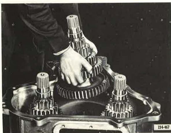
Figure 20. Installing Front Countershaft Assembly
