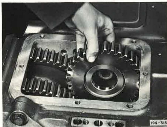
Figure 34. Installing Fourth Speed Gear
