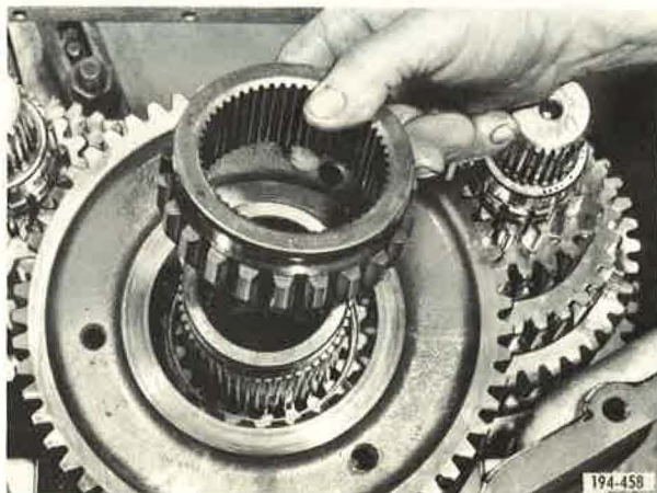
Figure 13. Removing First Speed Sliding Clutch
