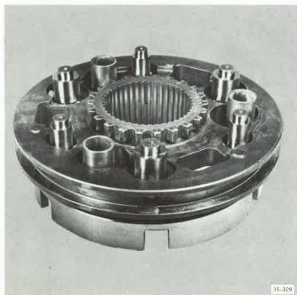
Figure 187. Support Tubes Installed
