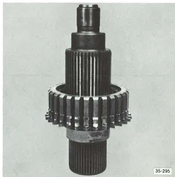
Figure 227. Lo-Range Gear Hub Installed on Shaft
