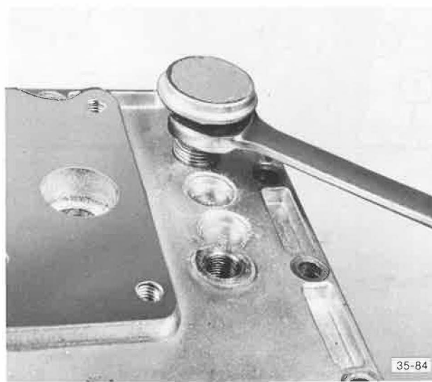
Figure 72. Removing Breather Vent
