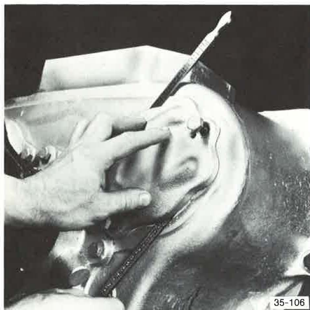
Figure 367. Measurement with Tapered Feeler Gauges
