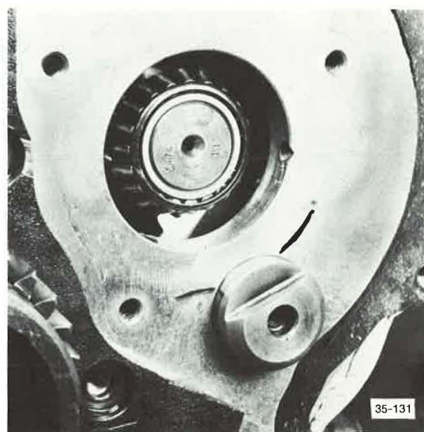
Figure 340. Reverse Idler Shaft Properly Aligned
