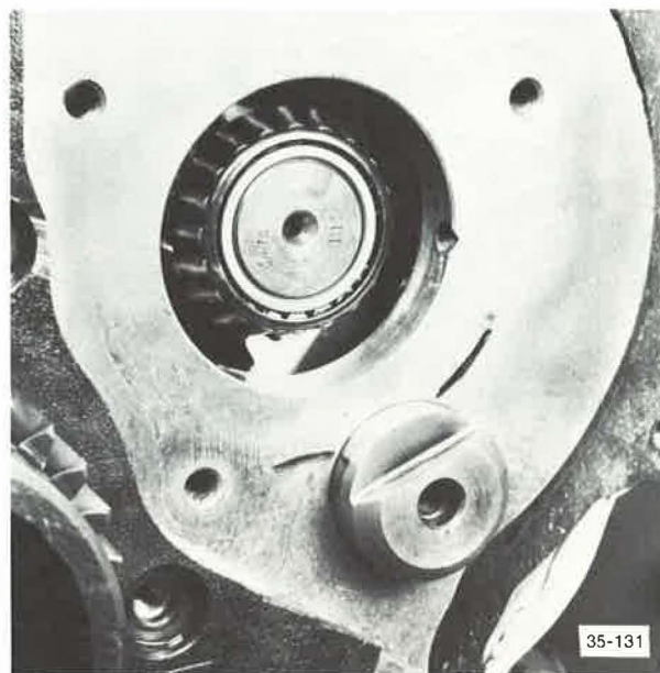
Figure 195. Reverse Idler Shaft Properly Aligned
