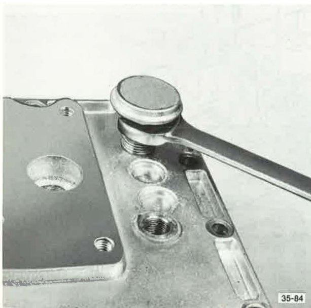
Figure 295. Installing Breather Vent
