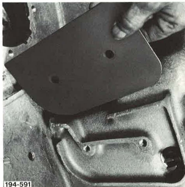
Figure 5. Magnetic Oil Filter Viewed from Inside Case
