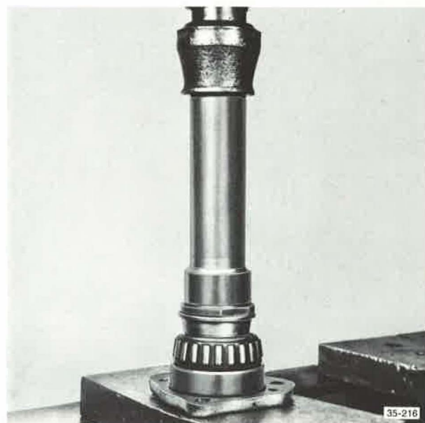
Figure 218. Pressing on Bearing
