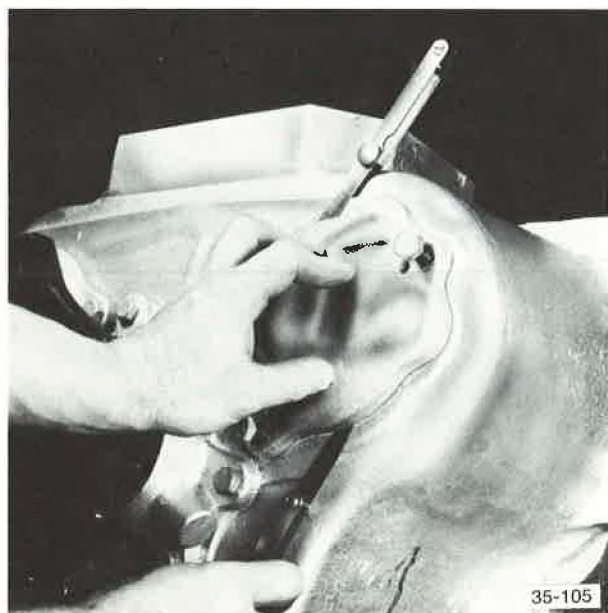
Figure 368. Measurement with Standard Feeler Gauges
