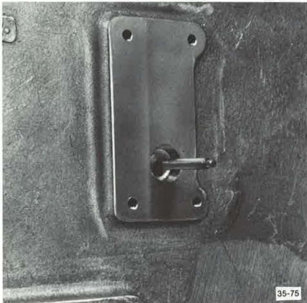
Figure 325. Interlock Plunger Installed
