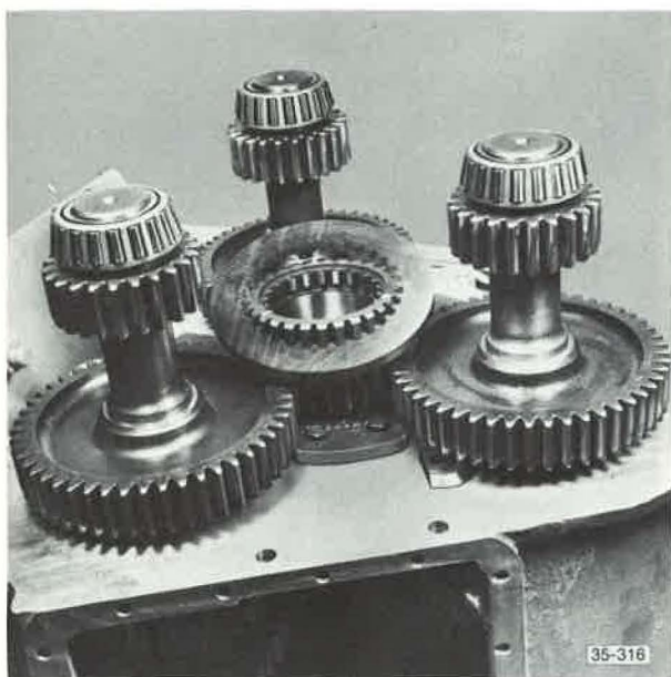
Figure 353. Installing Main Drive Gear Drive Plate
