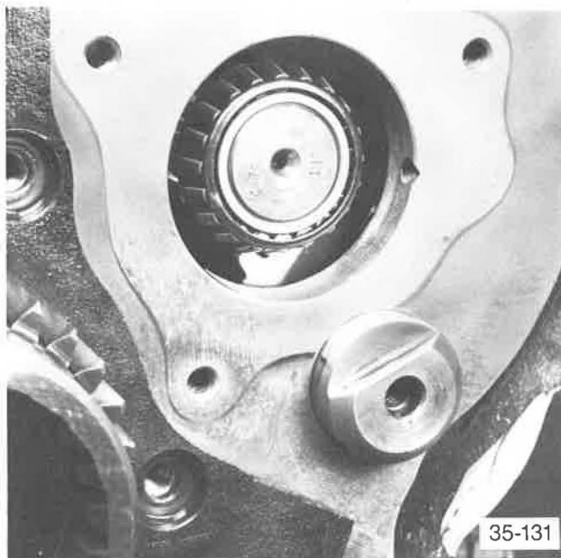
Installing Reverse Idler Shaft
