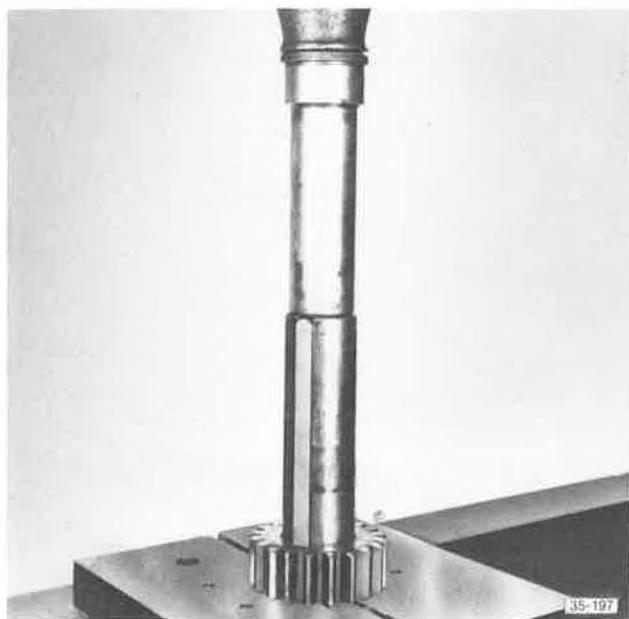
Pressing Second Speed Gear Off Of Shaft
