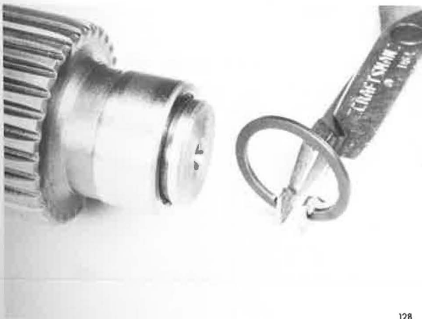
Removing Front Bearing Race Snap Ring
