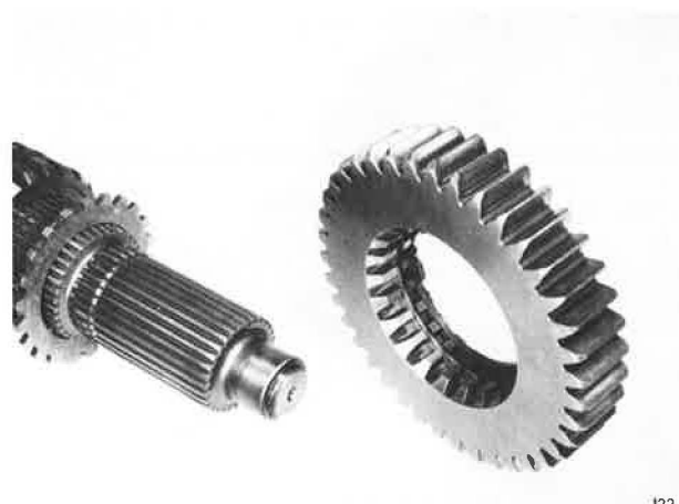
Removing Third Speed Gear
