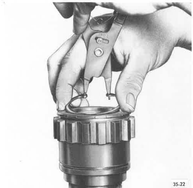
Removing Spigot Bearing Snap Ring
