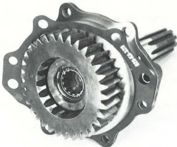
Removing Gasket From Main Drive Pinion Assembly
