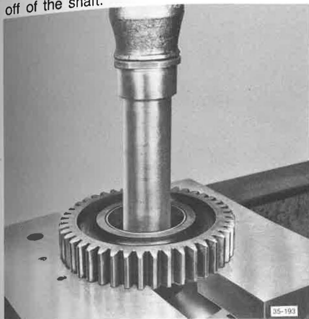
Pressing Main Drive Gear Off Of Shaft
