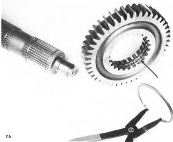
Removing Snap Ring From Second Speed Gear
