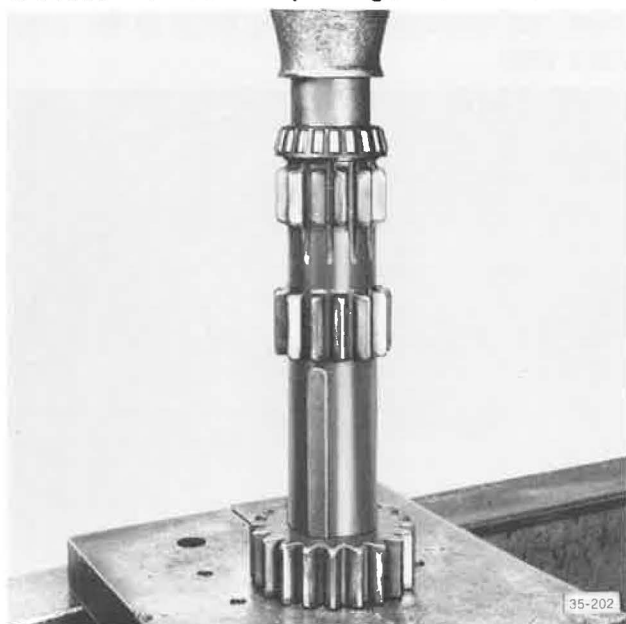
Pressing Second Speed Gear Onto Shaft
