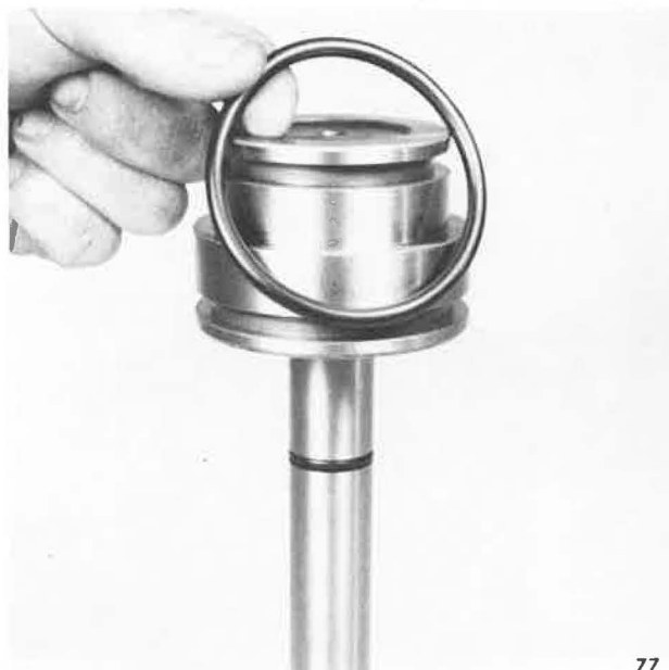
Removing O-Ring From Middle Of Piston
