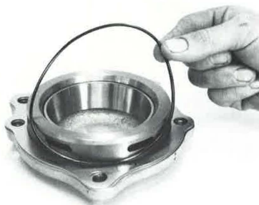
Removing O-Ring From Cover
