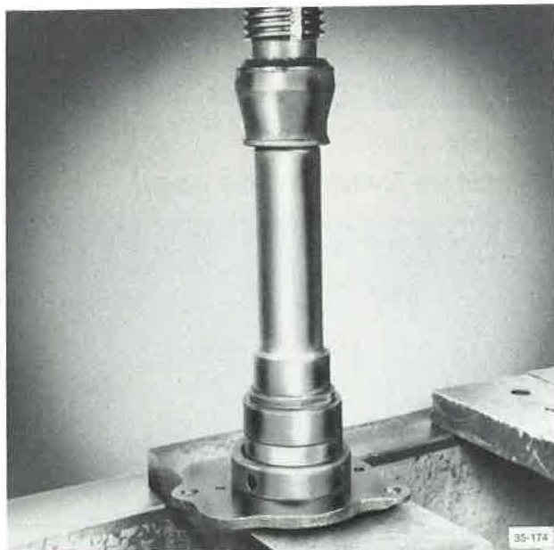
Pressing Front Bearing Outer Race Into Cover
