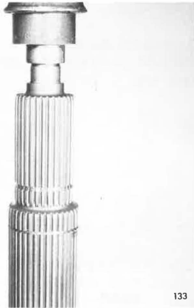
Pressing Bearing Inner Race Onto Front Of Mainshaft
