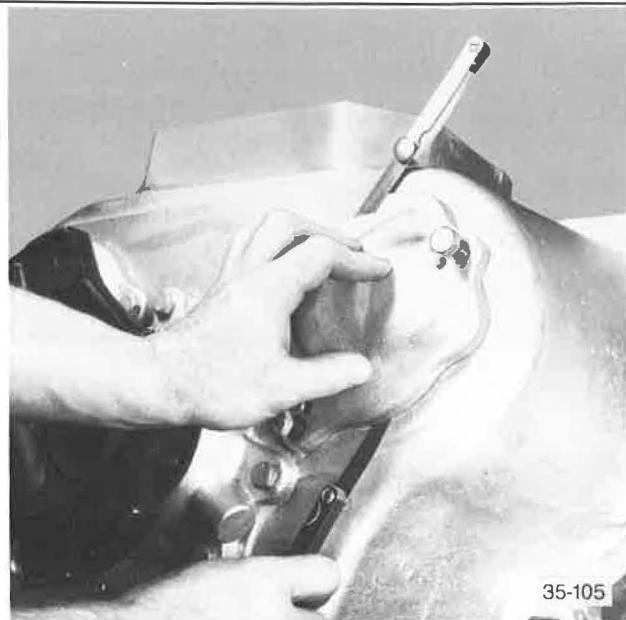
Measuring With Standard Feeler Gauges
