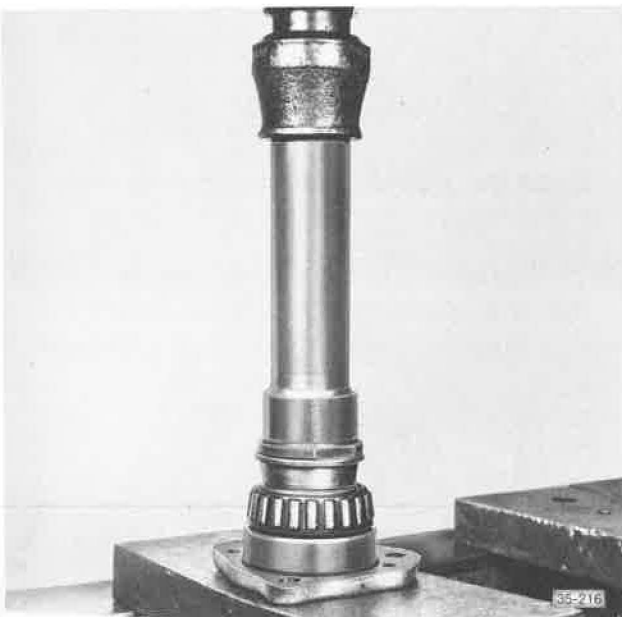
Pressing Bearing Onto Front Cover
