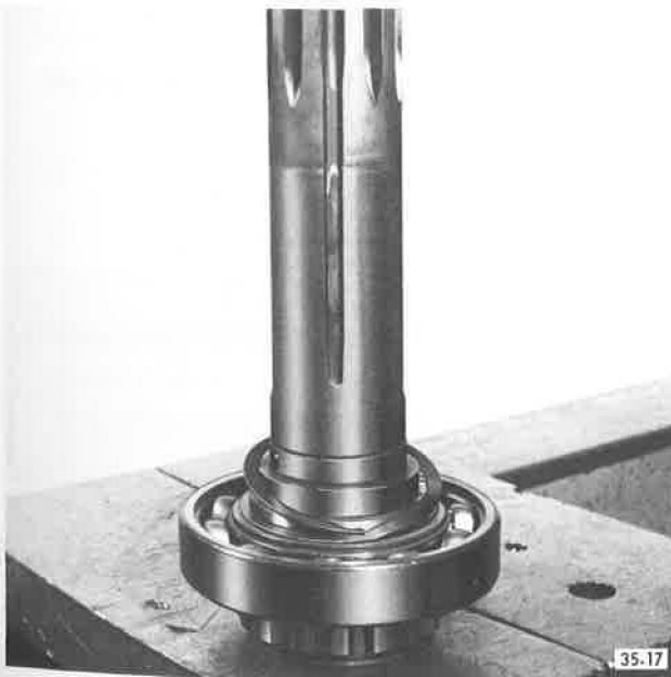
Removing Spiral Snap Ring
