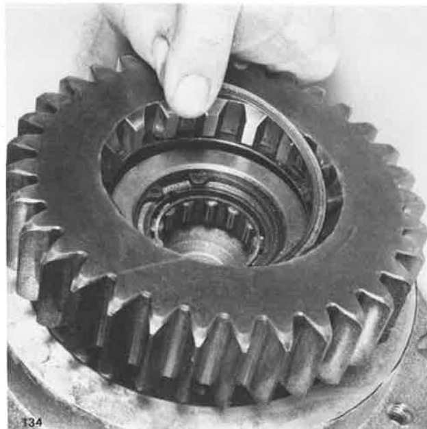
Installing Spiral Snap Ring
