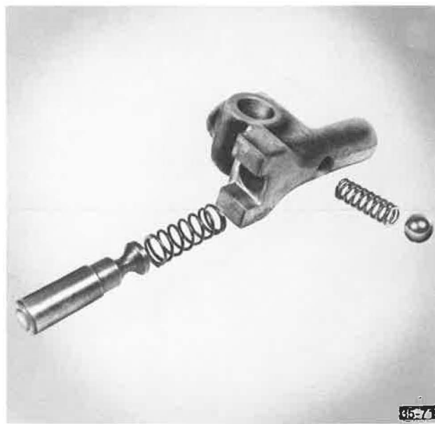
Disassembly Of First/Reverse Shifter
