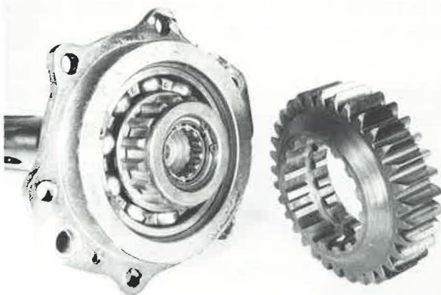
Removing Main Drive Pinion Gear From Shaft
