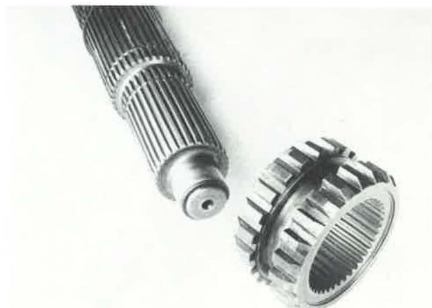
Installing Second/Third Speed Sliding Clutch
