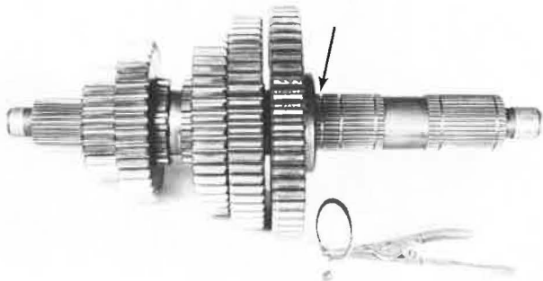
Removing Snap Ring Behind Reverse Gear
