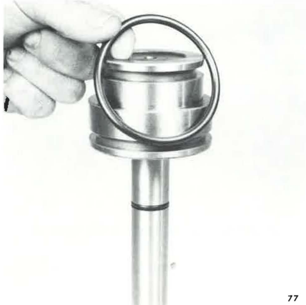
Installing O-Ring Onto Middle Of Piston
