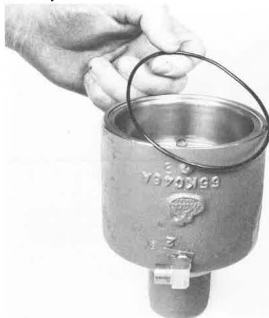
Removing O-Ring From Cylinder
