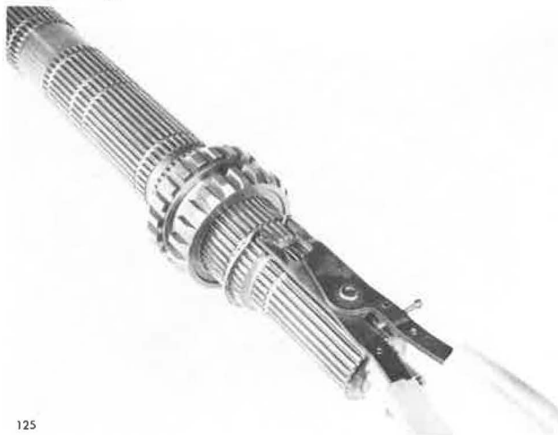
125 Removing Mainshaft Third Speed Gear Snap Ring
