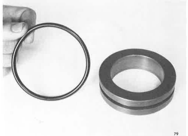
Installing O-Ring Onto Shift Sleeve
