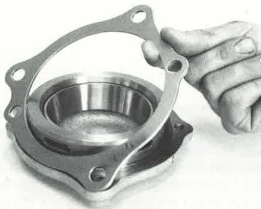
Installing Shim Pack Onto Rear Bearing Cover
