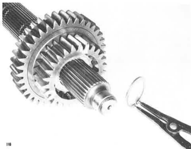
Removing Mainshaft Snap Ring From Inside Fifth Speed Gear
