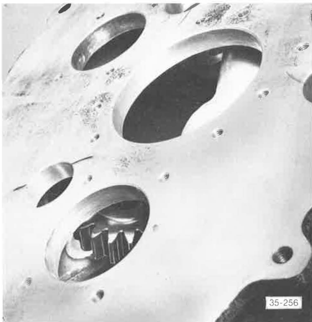
Installing Reverse Idler Gear
