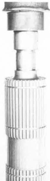
Pressing Bearing Inner Race Onto Rear Of Mainshaft
