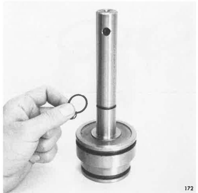
Installing O-Ring Onto Shift Rail
