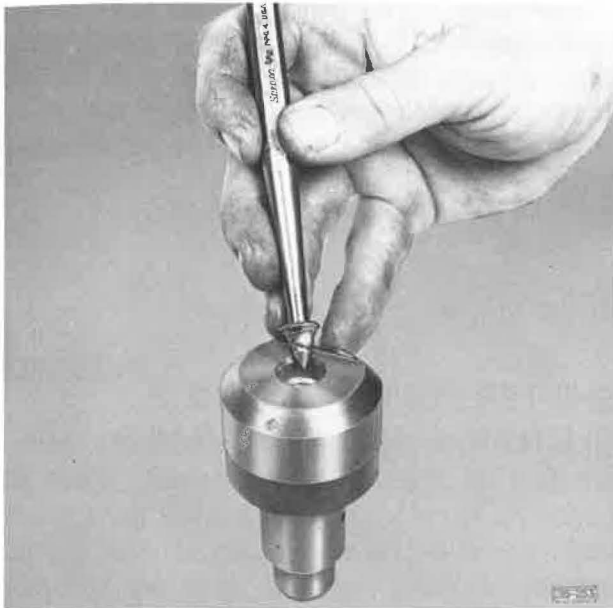
Removing Expansion Plug
