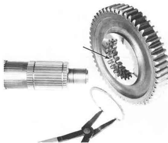
114 Removing Snap Ring From First Speed Gear
