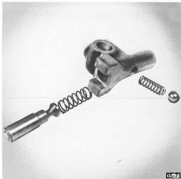
Reassembly Of First/Reverse Shifter
