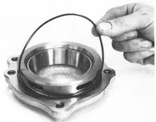
Installing O-Ring Onto Cover
