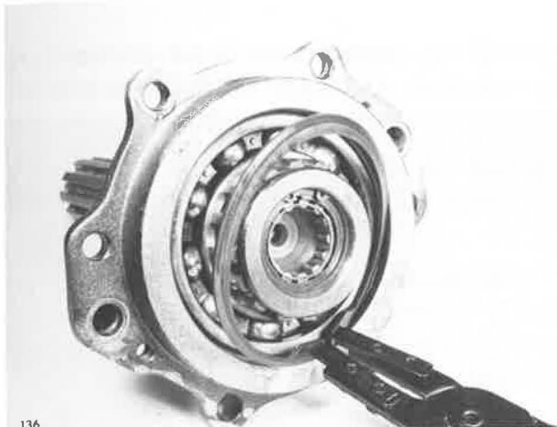
Installing Snap Ring Into Cover
