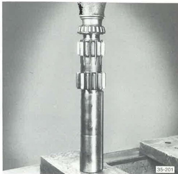
Pressing Rear Bearing Onto Shaft
