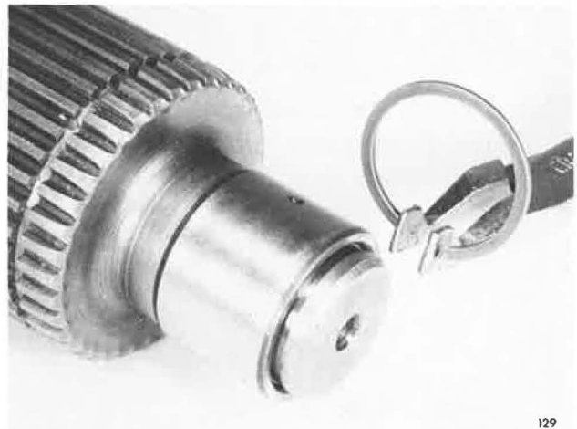
Installing Rear Bearing Inner Race Snap Ring
