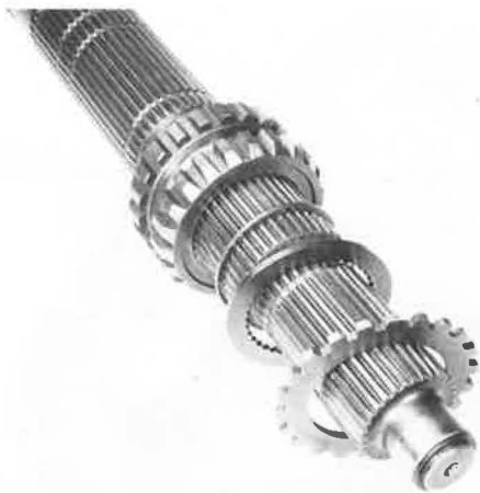
124 Removing External And Internal Tooth Thrust Washers
