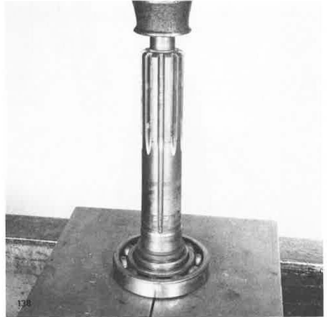
Pressing Bearing Off Of Shaft
