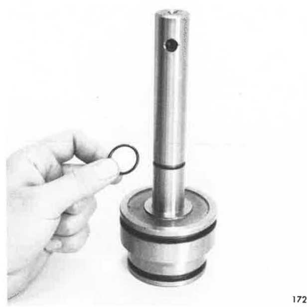
Removing O-Ring From Piston Shift Rail
