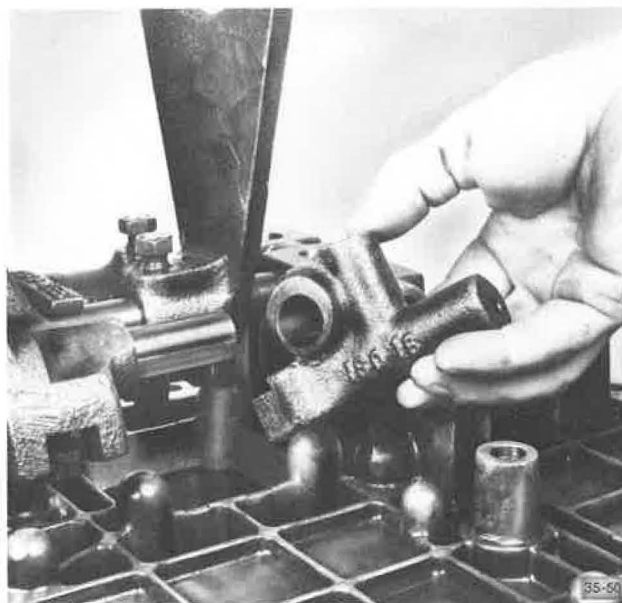
Installing First/Reverse Shifter
