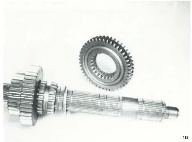
Installing Second Speed Gear Onto Mainshaft
