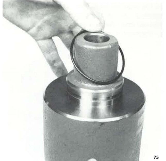
Installing O-Ring Onto Cylinder
