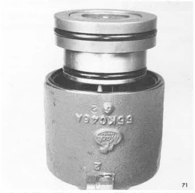
Installing Piston Assembly Into Cylinder
