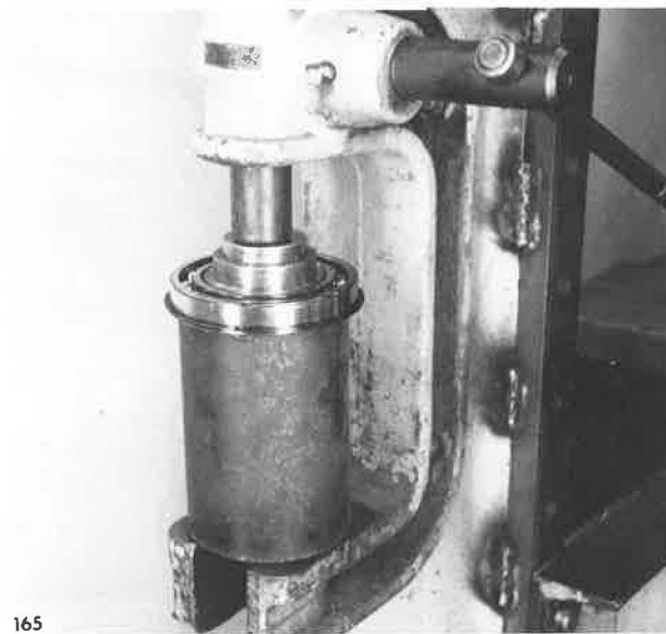
Pressing Sleeve Out Of Bearing
