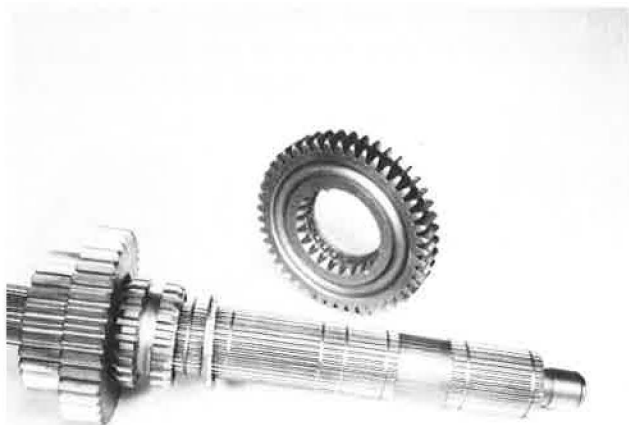
Removing Second Speed Gear
