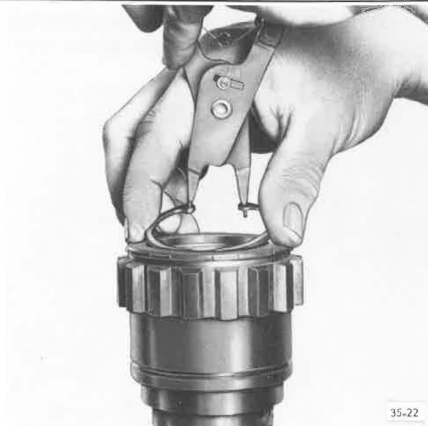
Installing Snap Ring Into Main Drive Pinion Shaft
