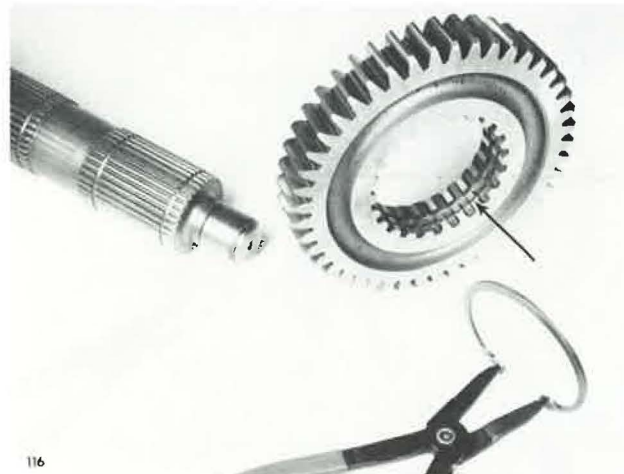
Installing Snap Ring Into Second Speed Gear
