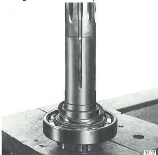
Installing Snap Ring Onto Main Drive Pinion Shaft
