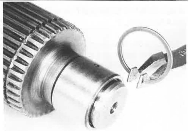
Removing Rear Bearing Race Snap Ring
