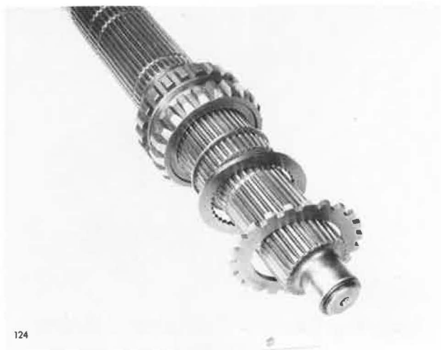
Installing Internal And External Tooth Thrust Washers
