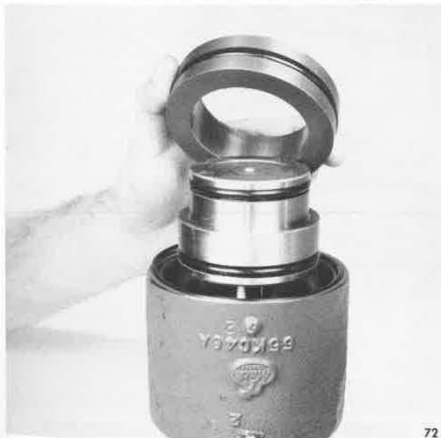
Installing Sleeve Onto Piston
