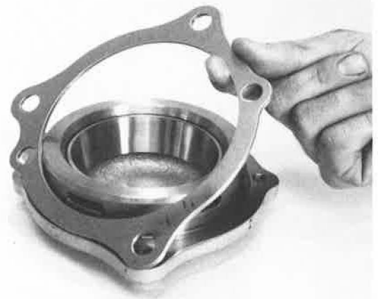
Installing Shim Pack Onto Cover
