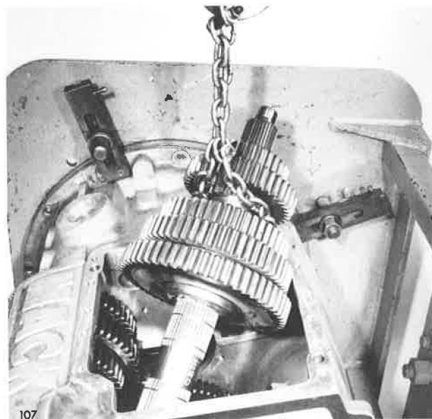
Removing Mainshaft Assembly From Case
