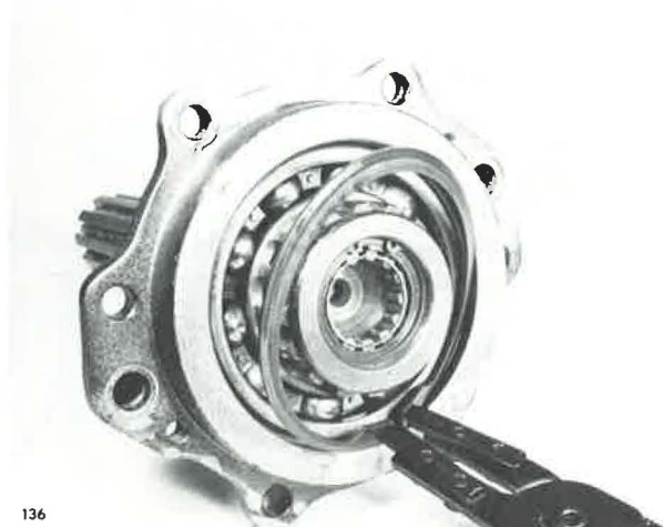
Removing Snap Ring From Cover
