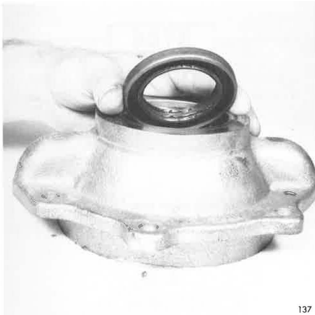
Removing Oil Seal From Cover
