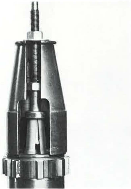
Removing Spigot Bearing
