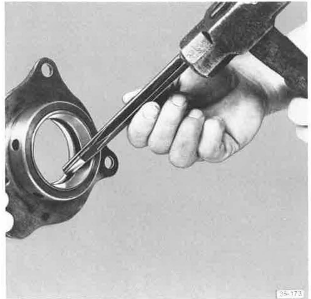
Removing Rear Bearing Race
