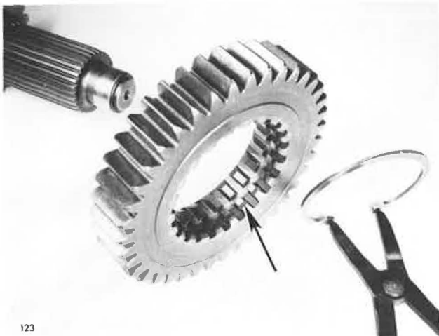
123 Removing Snap Ring From Third Speed Gear
