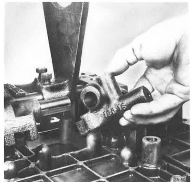
Removing First/Reverse Shifter
