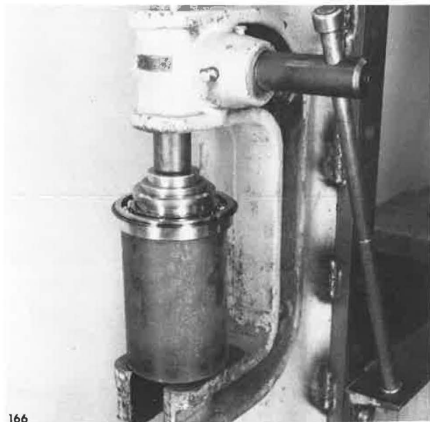
Pressing Sleeve Into Bearing
