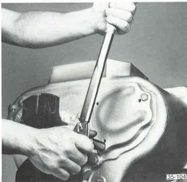
Tightening Capscrews In Rear Bearing Cover
