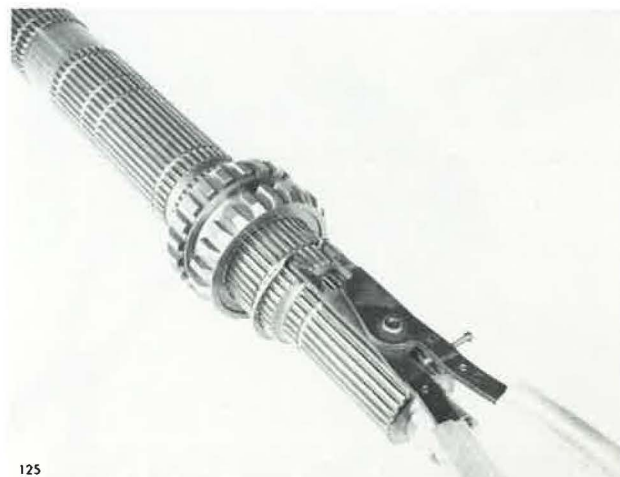
Installing Third Speed Gear Snap Ring
