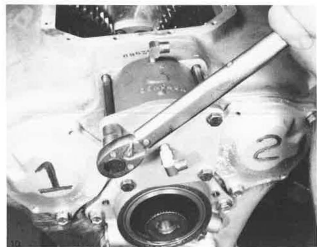
Tightening Shift Cylinder Capscrews
