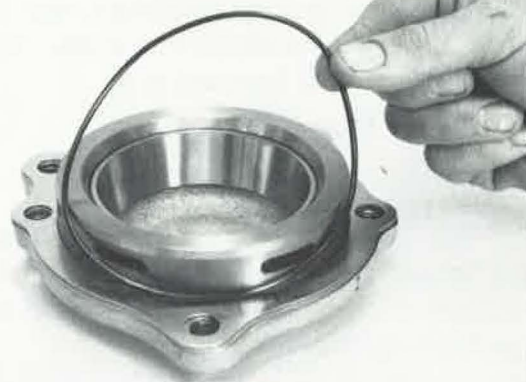
Installing O-Ring Onto Rear Bearing Cover
