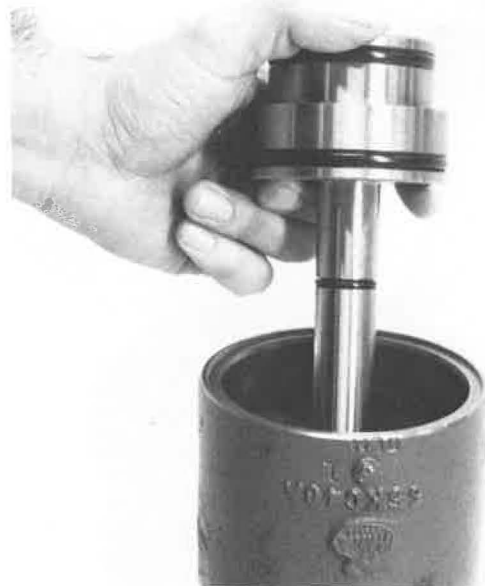
Removing Piston From Cylinder
