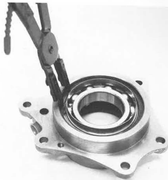
Removing Bearing Retaining Snap Ring
