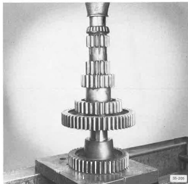
Pressing Main Drive Gear Onto Shaft
