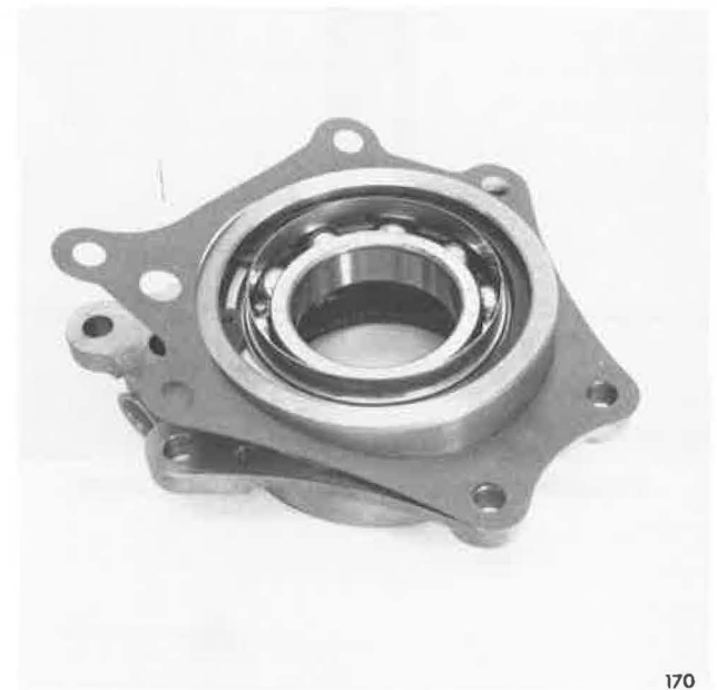
Installing Gasket Onto Cover
