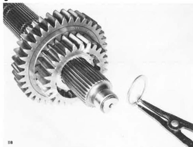
Installing Mainshaft Fifth Speed Gear Snap Ring
