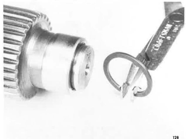
Installing Front Bearing Inner Race Snap Ring
