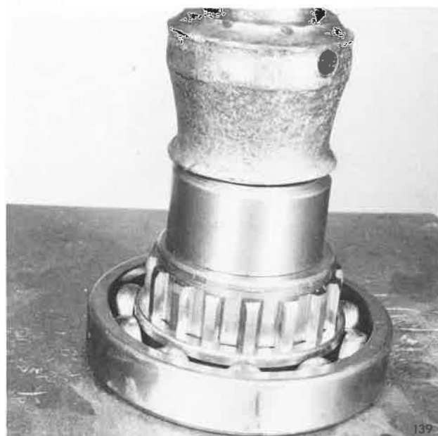
Pressing Bearing Onto Main Drive Pinion Shaft
