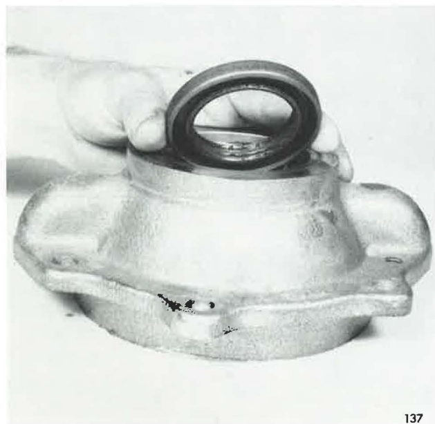
Installing Oil Seal Into Cover
