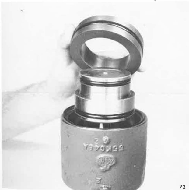
Removing Sleeve From Piston
