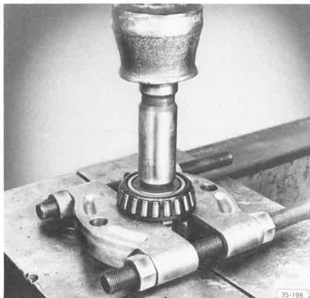
Pressing Off Rear Bearing
