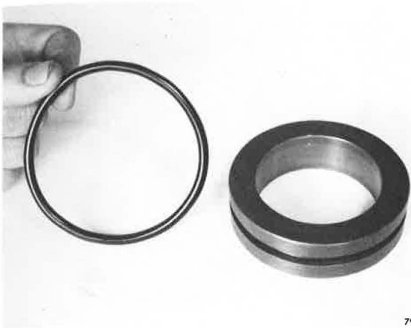
Removing O-Ring From Sleeve
