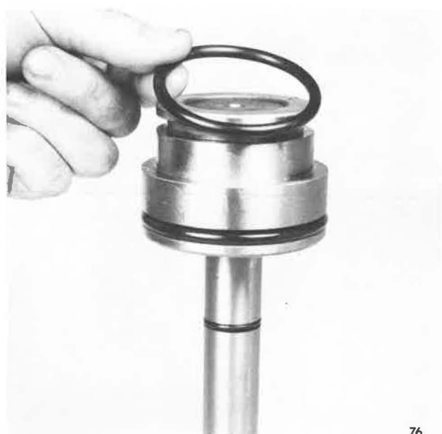
Removing O-Ring From Rear Of Piston
