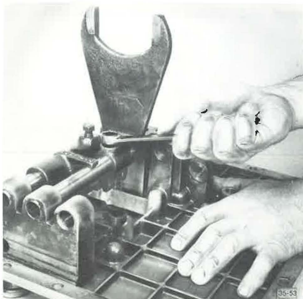
Removing Setscrew From Second/Third Shift Fork
