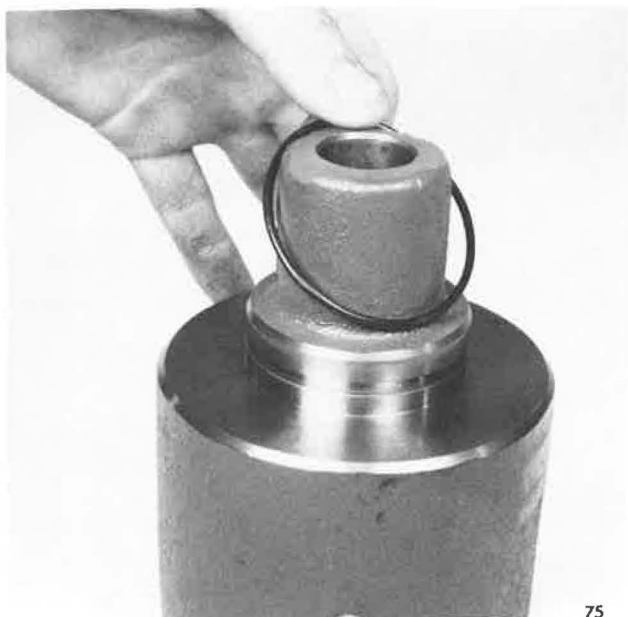
Removing O-Ring From Cylinder
