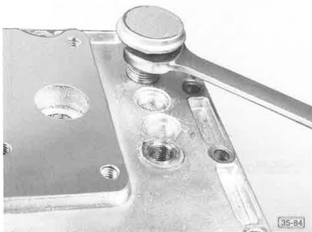
Installing Breather Vent
