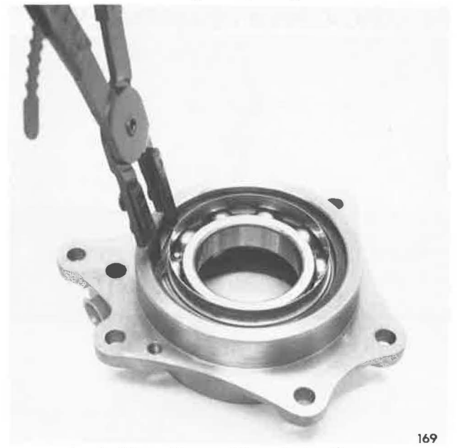
Installing Snap Ring Into Cover
