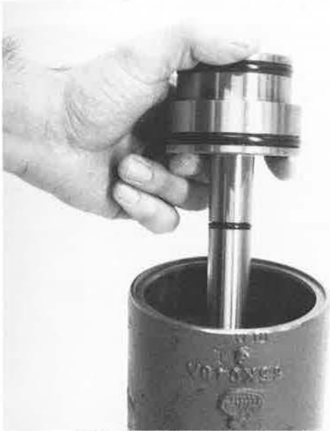
Installing Piston Into Cylinder
