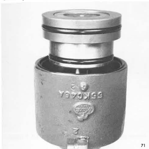
Piston Assembly Partially Removed
