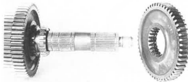
Removing Reverse Gear From Mainshaft
