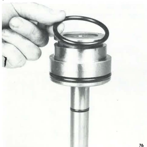
Installing O-Ring Onto Rear Of Piston
