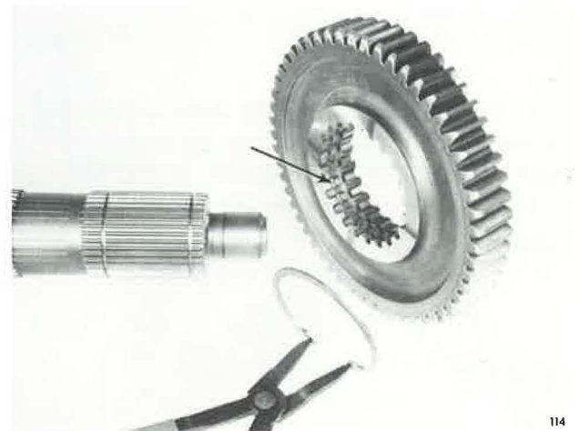
Installing Snap Ring Into First Speed Gear
