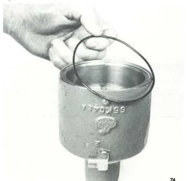
Installing O-Ring Into Cylinder
