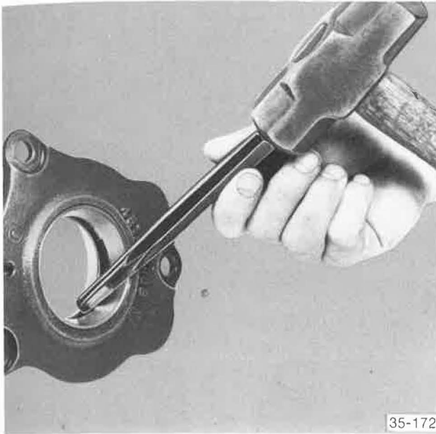
Removing Front Bearing Race
