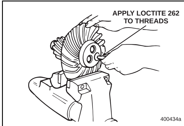
Figure 211 — Applying Loctite 262 to Capscrew Threads
