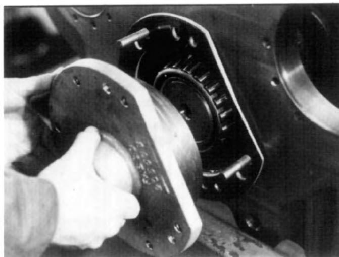
FIG. 6.1-13 Press smaller bearing cup into end cap. Using approximately .150 inches pile of shims, assemble end cap to front of housing. Extended length bolts with the heads removed can be used as simple guides to support and locate all gaskets, shims and end caps as required.
