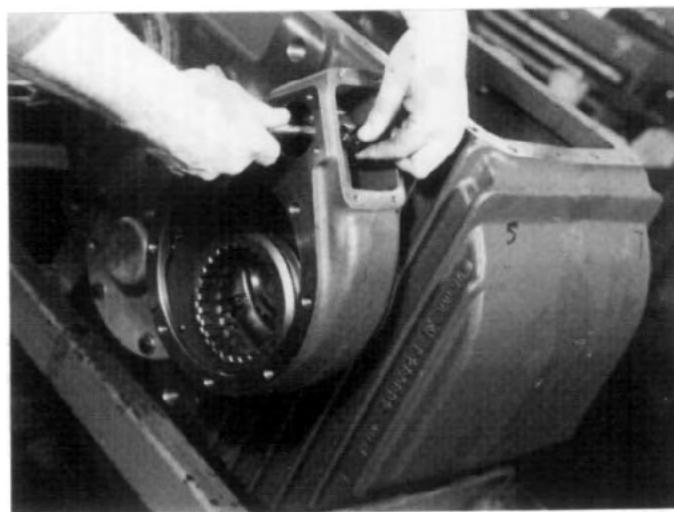
FIG. 6.7-4 If not already mounted, assemble declutch housing to transfer case housing. If not already completed, transfer case shaft end float must be adjusted at this point. Assemble shift fork in clutch collar groove and place in declutch housing. Slide shift shaft into shift fork and add pinch bolts.
