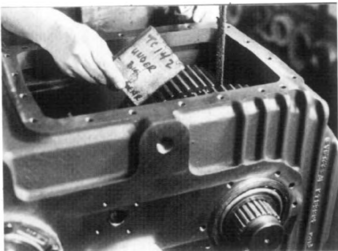
FIG. 6.4-8 Remove wooden block from under gear.
