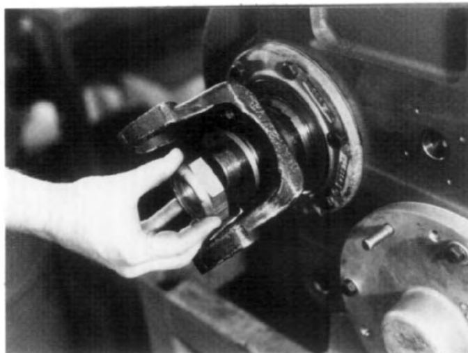
FIG. 5.1-3 Remove yoke or companion flange and seal carrier from upper shaft.
