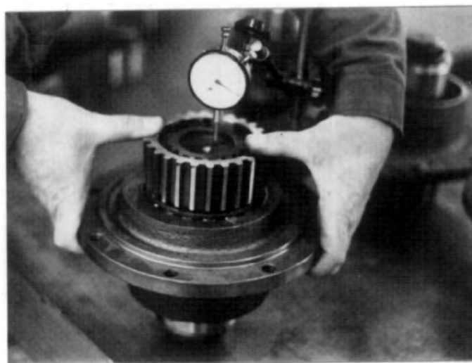
FIG. 6.7-3 Add blanking sleeve or yoke, washer and locknut to output shaft and tighten nut. Mount magnetic base dial test indicator to flange of carrier and check for bearing float on end of shaft as indicated in End Float Adjustment section. End float should be between .003 and .008 inches. Spacer between bearing cones must be machined or changed to one of suitable dimensions to provide the correct end float dimension.
