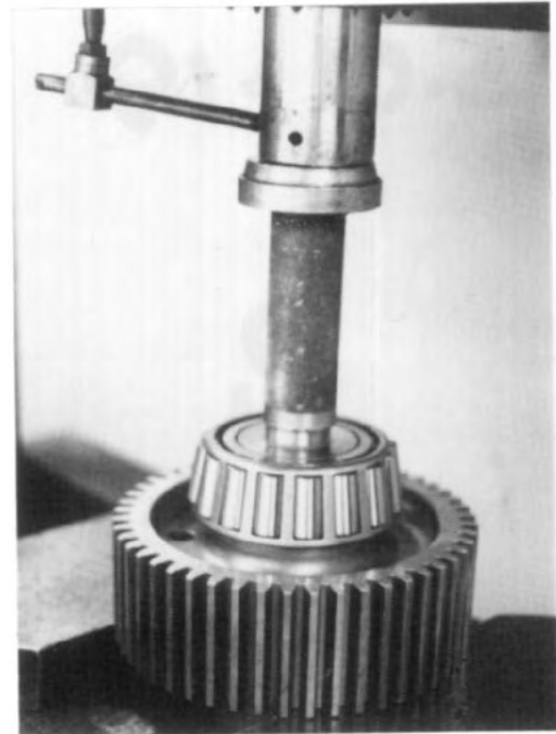
FIG. 5.1-19 Use suitable hydraulic press to disassemble shaft from intermediate gear.
