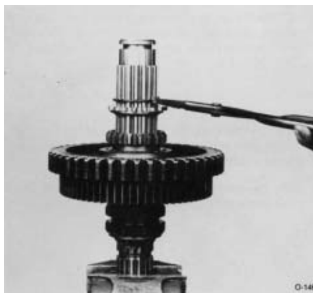
15. Install snap ring in snap ring groove at rear of mainshaft.
