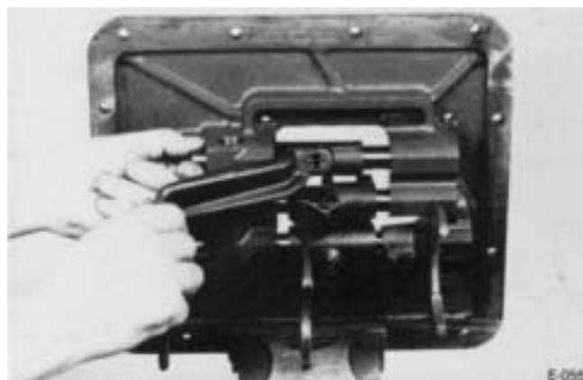
8. Install the 4th-5th speed shift bar in upper bore in housing installing shift yoke on bar, fork to the front.
