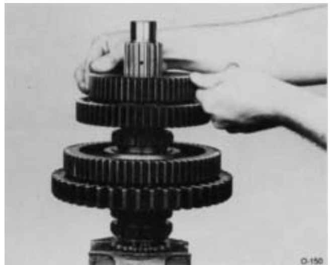
19. Install 4th speed gear, clutching teeth up, against 3rd speed gear.
