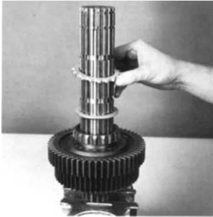
12. Install the spacer on shaft against washer.
