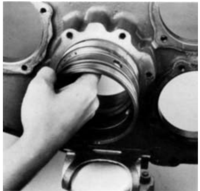
8. Remove the two bearing cups and outer spacer from bore in auxiliary plate.
