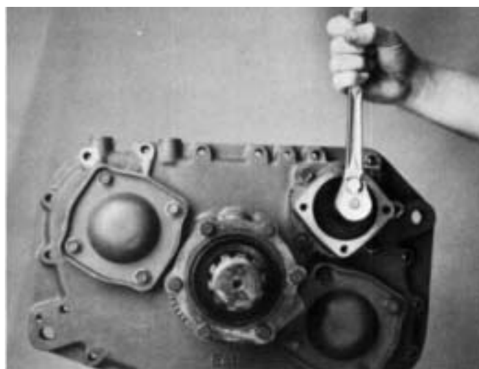
2. Remove nut from end of yoke bar.
