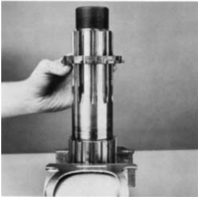
5. Remove the splined spacer from output shaft.
