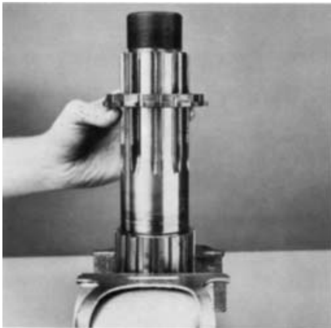
5. Remove the splined spacer from output shaft.
