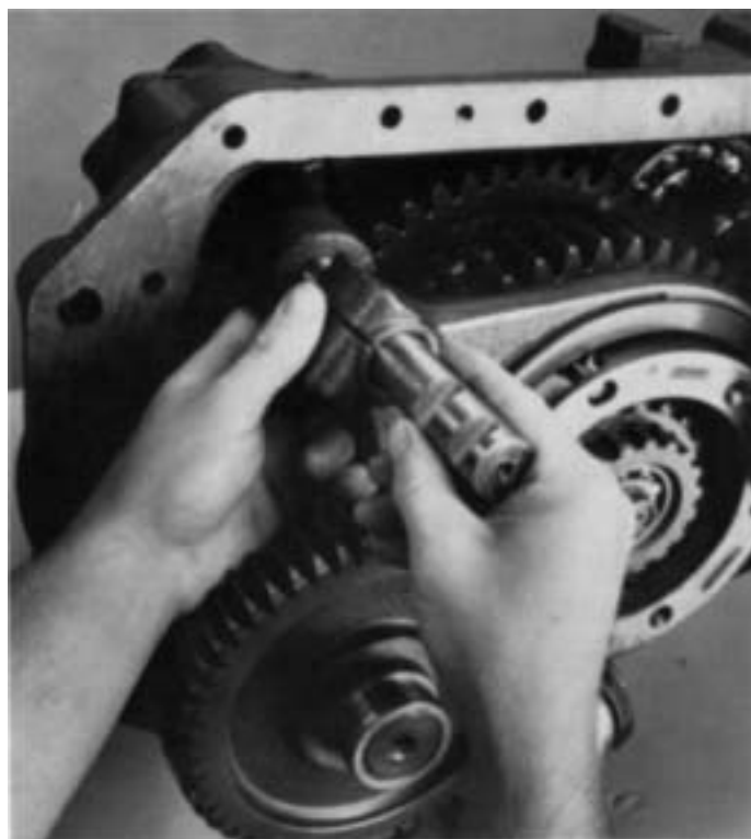
4. Pull yoke bar from bore of cylinder housing.
