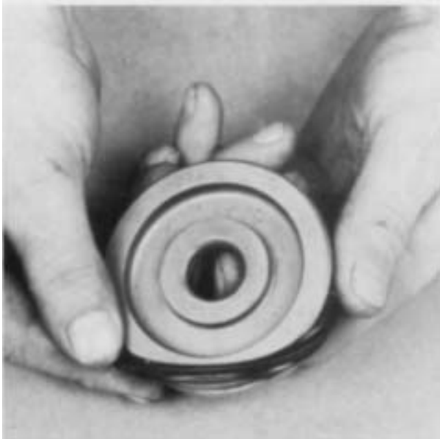
5. Remove the O-rings from the piston.
