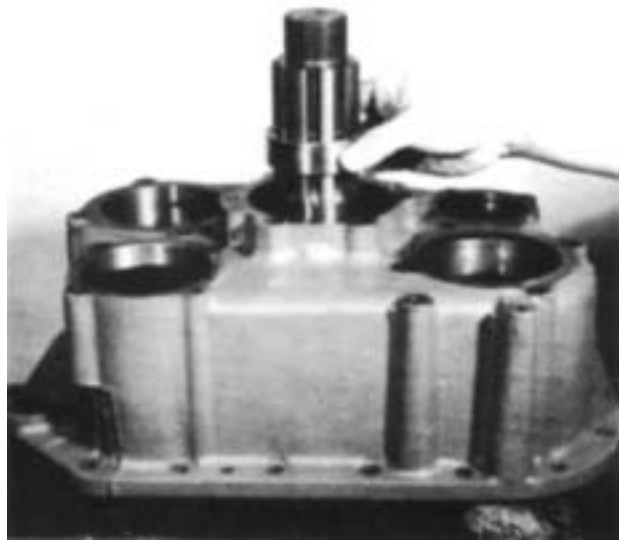
9. Install the bearing inner spacer on the shaft and against the front bearing cone.
