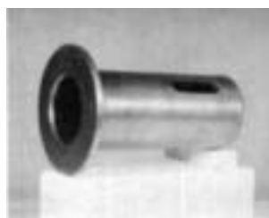
BEARING DRIVERS Print Number T-18042 (Dimensions for all drivers necessary on this print.) Used to install bearings on shafts and in bores.
