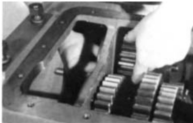
3. Hold the gear and thrust washer in place in the case with the thrust washer between the gear and housing boss and the idler gear meshed with the teeth of the countershaft reverse gear. Insert the idler shaft through the bore in the rear case wall, the gear and washer and the housing boss. Make sure that the long hub of the gear faces towards the front of the case.
