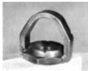
OUTPUT SHAFT HANGER BRACKET Make from yoke stop nut and flat steel stock Used to support the auxiliary section when installed or removed from the front case in the vertical position.
