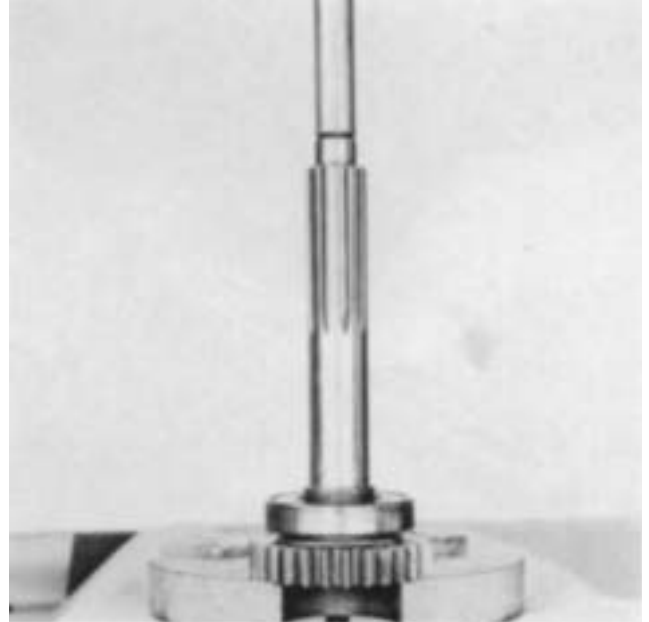
6. Using the rear face of the drive gear as abase, press the shaft through the gear to unseat the bearing from the shaft. This will free the bearing, spacer and drive gear. If necessary, remove the snap ring from the drive gear.
