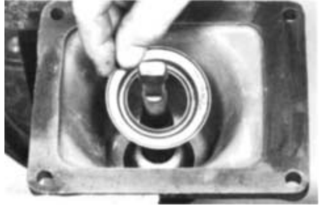
4. Install the tension spring washer in the housing.
