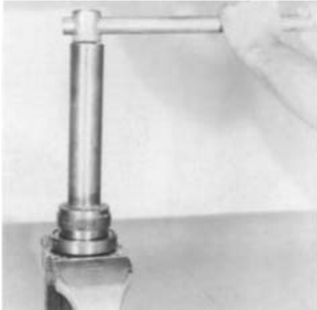
5. Turn the bearing nut from the shaft. (LH thread)
