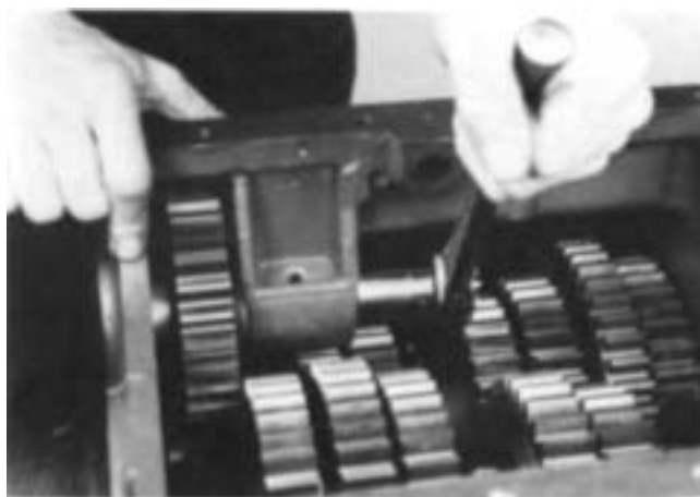
4. Secure the shaft with the washer and elastic stop nut.
