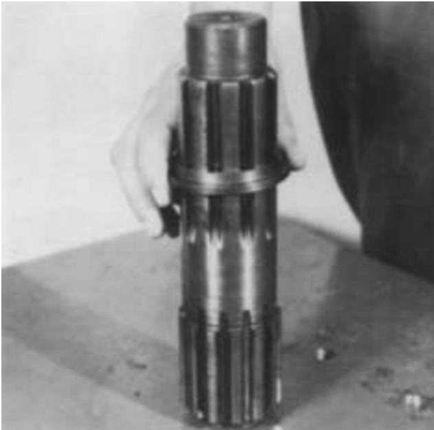
6. Remove the stepped washer from the shaft.
