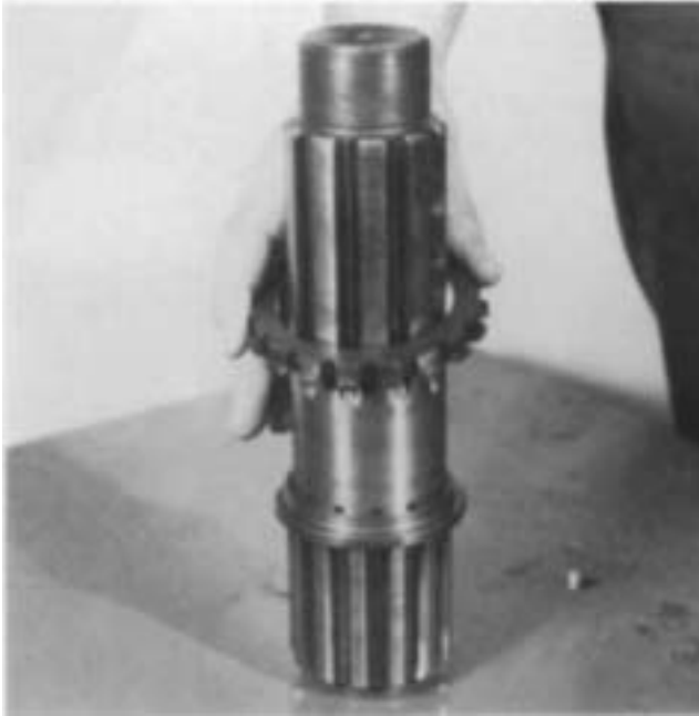
5. Remove the splined spacer from the shaft.
