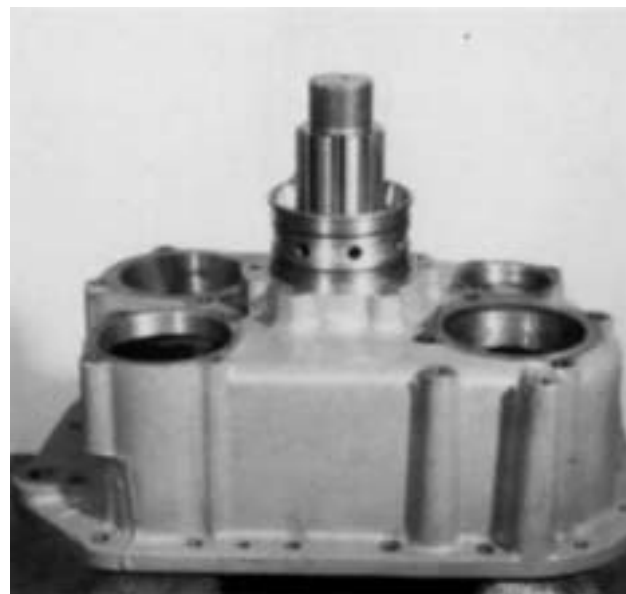
10. Stack the two bearing cups and outer spacer in the output shaft bore in the proper sequence. Make sure that the front bearing cup taper matches the taper direction off the front bearing cone.
