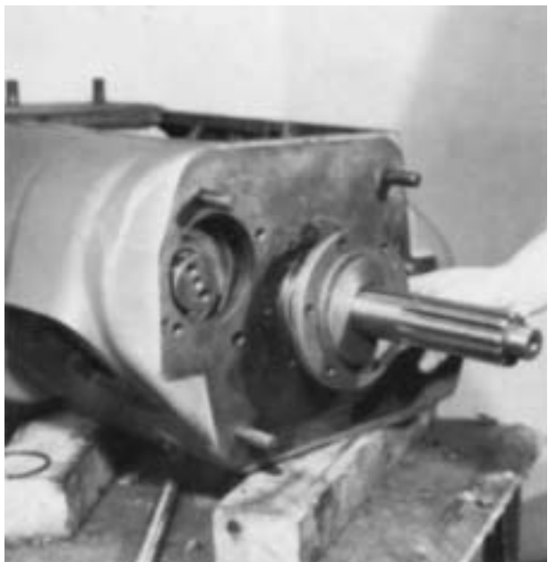
1. Remove the front bearing cover.
