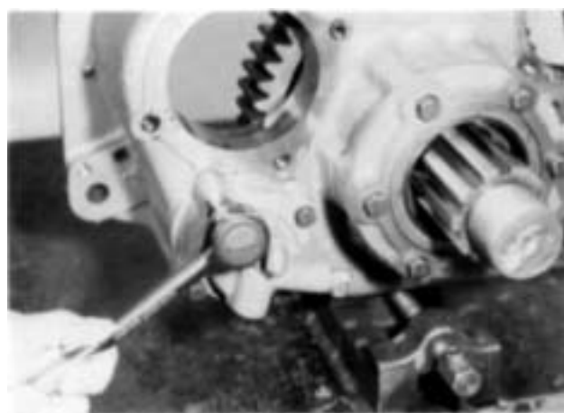
1. Remove the shift cylinder cover.
