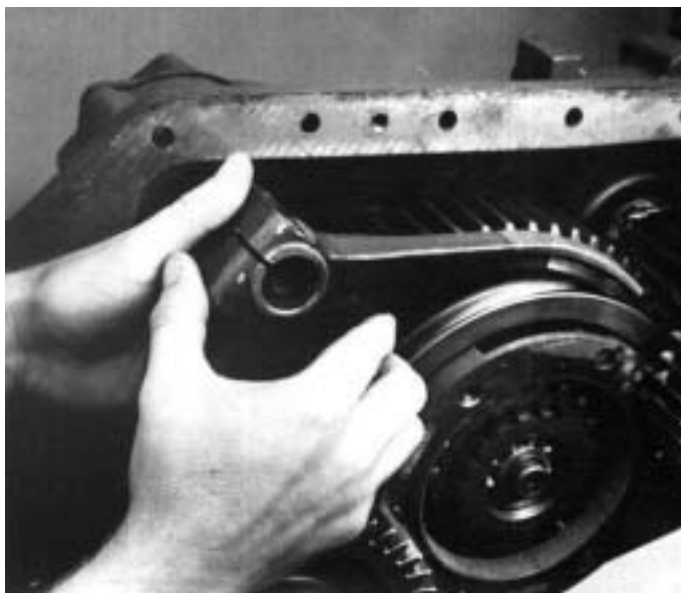
5. Remove range yoke from sliding clutch of synchronizer assembly.
