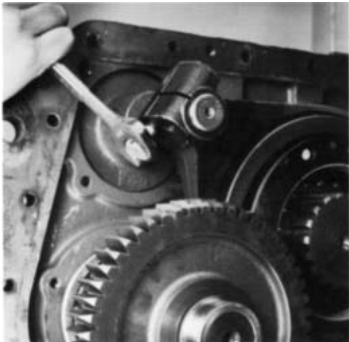
3. Cut lockwire and remove two yoke lockscrews.
