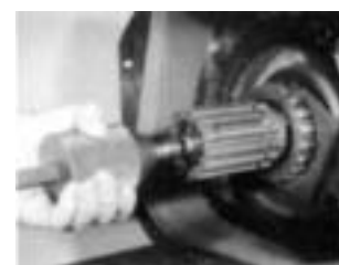
SNAP RING INSTALLER Print Number T-16552-1-N Used to install the snap ring in the output shaft quill. (RT-12515 Series)
