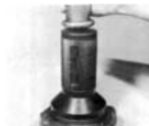
OIL SEAL DRIVER Print Number T-18088-23 Used to install the oil seal in the rear bearing housing.
