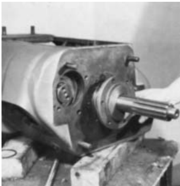
1. Remove the front bearing cover.
