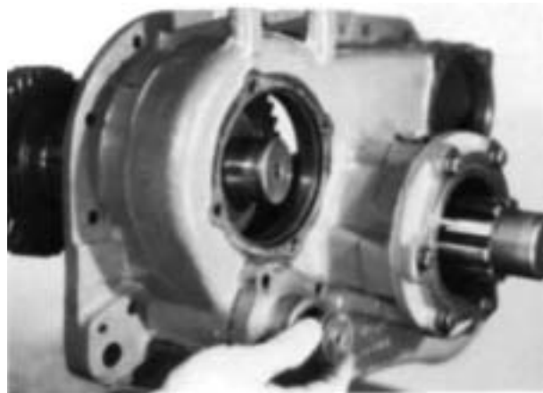
3. Pull the yoke bar from the cylinder housing; remove the O-ring if necessary.
