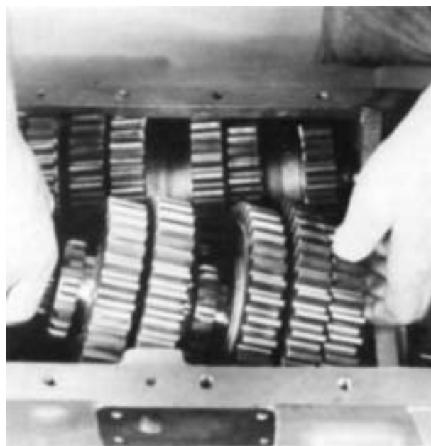
21. From inside the case, insert the rear of the mainshaft through the rear bearing bore and lower the assembly into position. Block the right countershaft against the side of the case and move the mainshaft pilot forward to seat in the pocket of the drive gear shaft.
