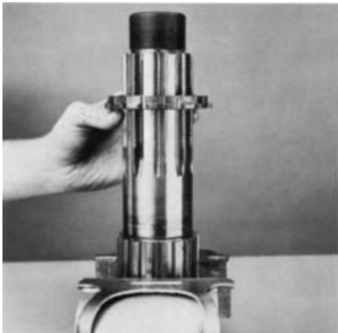
5. Remove the splined spacer from output shaft.
