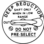
Lever to "IN" (Valve CLOSED)
