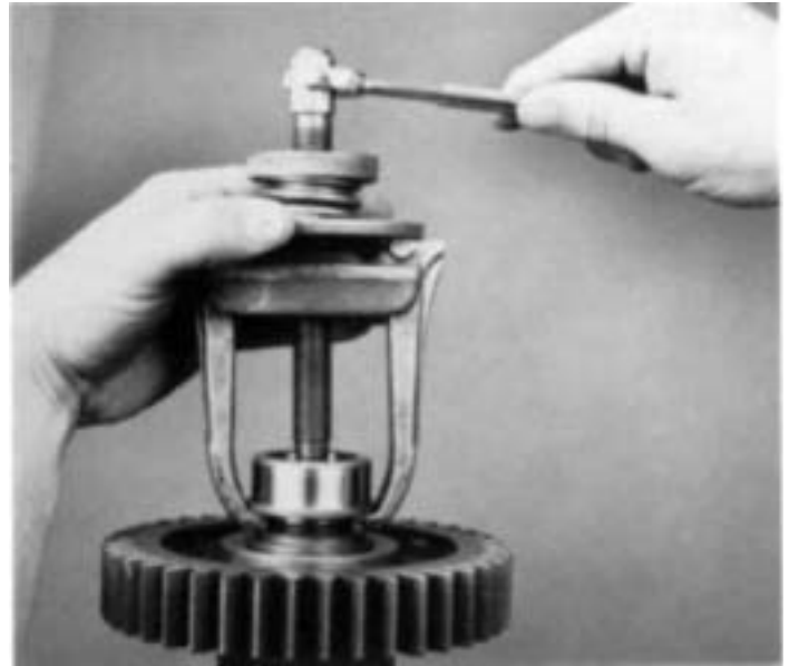
7. Remove bearing inner race from front of counter-shaft with jaw puller.
