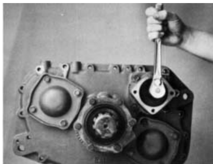
2. Remove nut from end of yoke bar.
