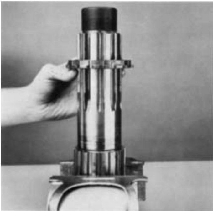
5. Remove the splined spacer from output shaft.
