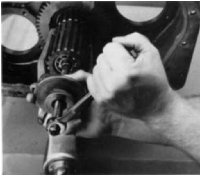
5. Remove range mainshaft with jaw puller.
