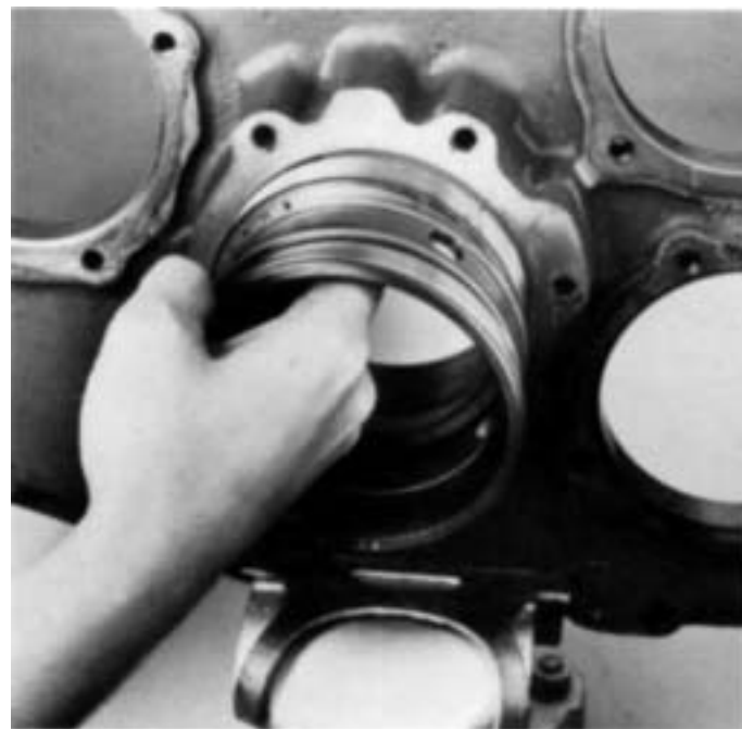
8. Remove the two bearing cups and outer spacer from bore in auxiliary plate.
