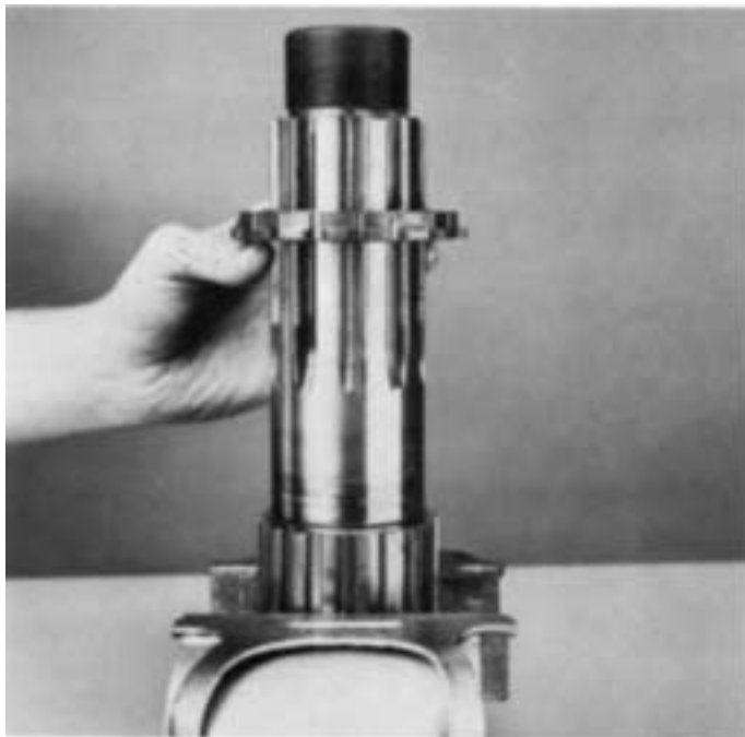
5. Remove the splined spacer from output shaft.
