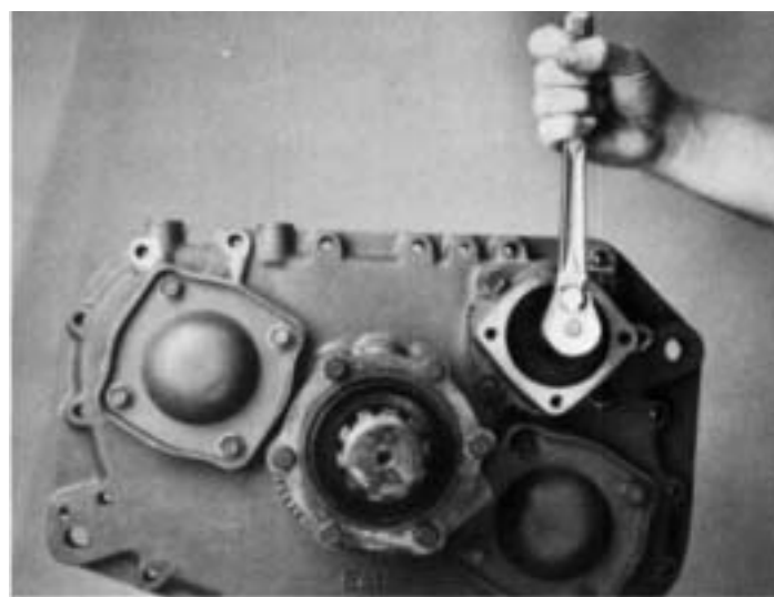
2. Remove nut from end of yoke bar.
