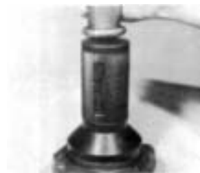
OIL SEAL DRIVER Print Number T-18088-37 Print Number T-18088-36 (RT-1110)
