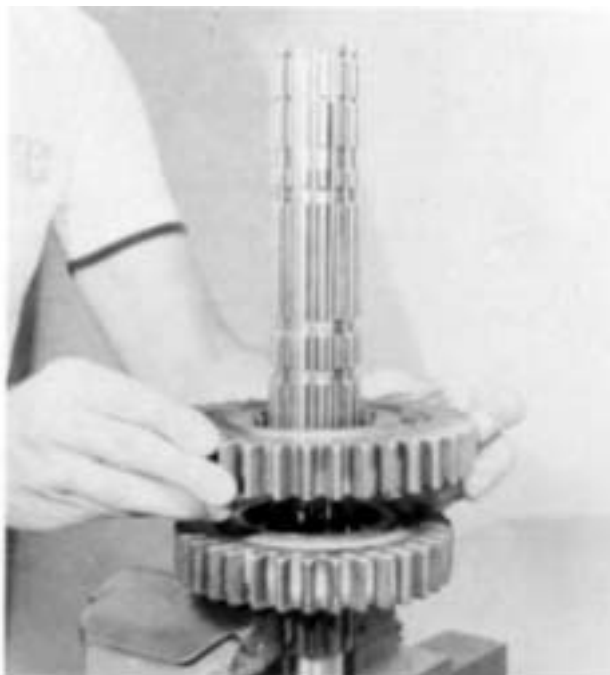
5. Install the second speed gear, clutching teeth up.
