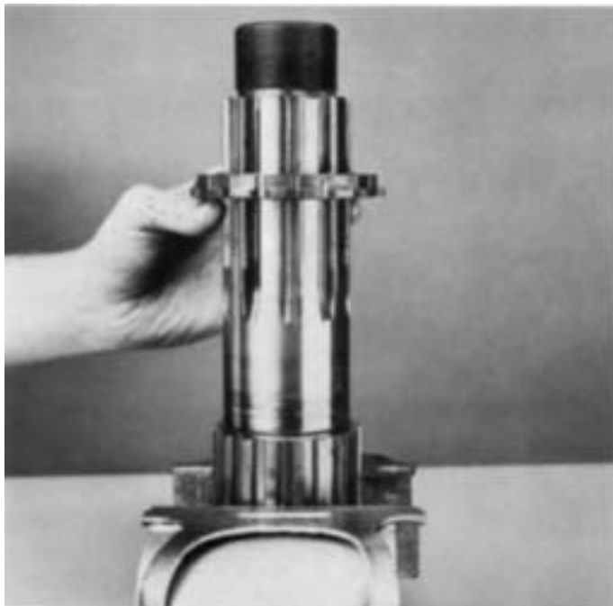
5. Remove the splined spacer from output shaft.
