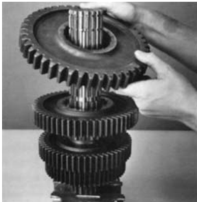
14. Install the LO speed gear on shaft against 1st speed gear, clutching teeth up.
