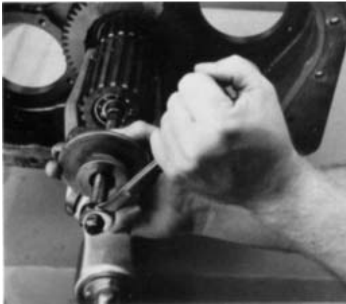
5. Remove range mainshaft with jaw puller.
