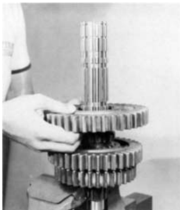
11. Install the first speed gear, clutching teeth down.
