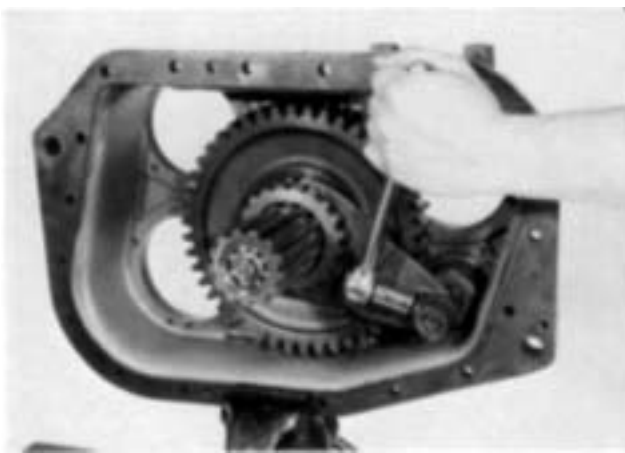
2. Cut the lockwire and turn out the lockscrew from the shift yoke.
