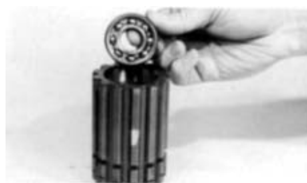
3. If necessary, remove the bearing from the mainshaft by tapping lightly from the inside with the range shift yoke bar or a similar size rod.
