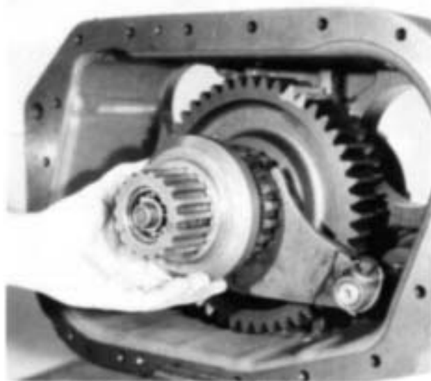
1. Install the coupler on the shaft, large diameter to the rear.
