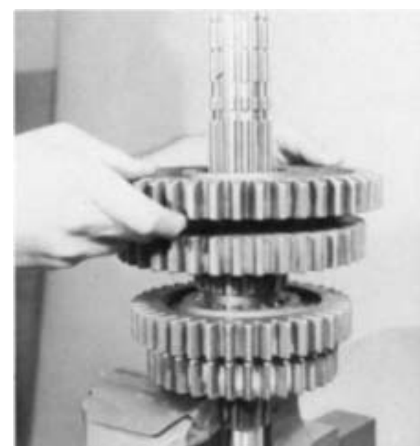
12. Install the low speed gear, clutching teeth up.
