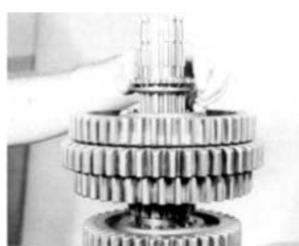
18. Install the spacer, flat surface down.
