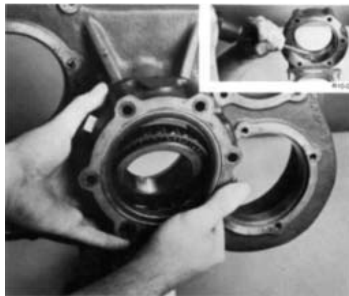
7. Turn out the capscrews and remove the rear bearing cover and gasket. The rear bearing cone will drop from bore in auxiliary plate when cover is removed. If necessary, remove the oil seal from cover (inset).
