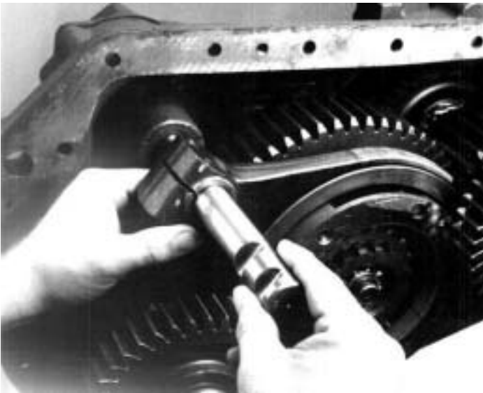
4. Pull yoke bar from bore of cylinder housing.
