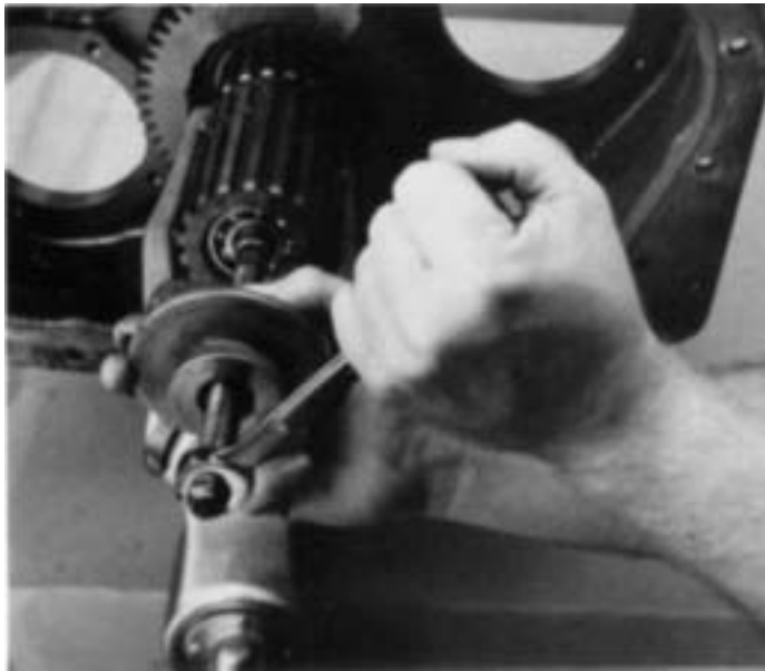
5. Remove range mainshaft with jaw puller.
