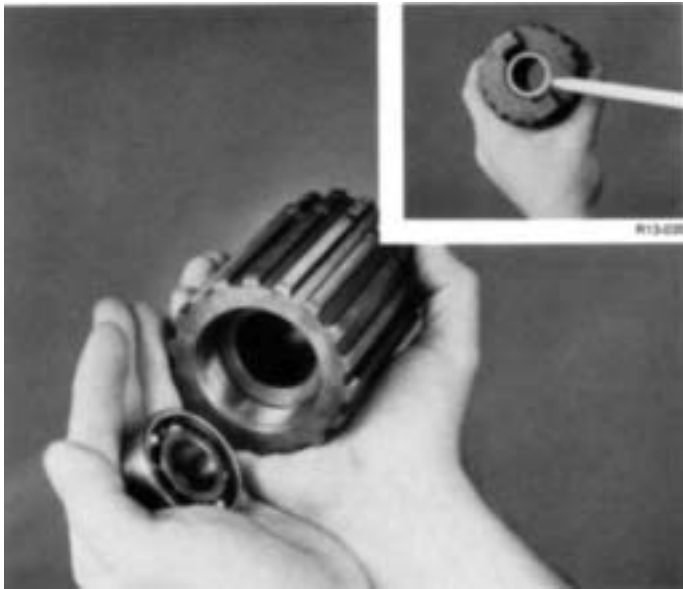
6. Remove bearing from front bore of mainshaft. If necessary, press bushing from mainshaft (inset).
