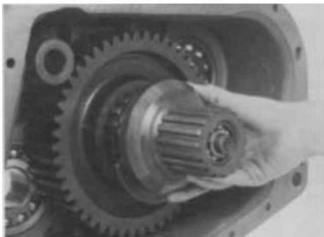
5. Slide the coupler off mainshaft.
