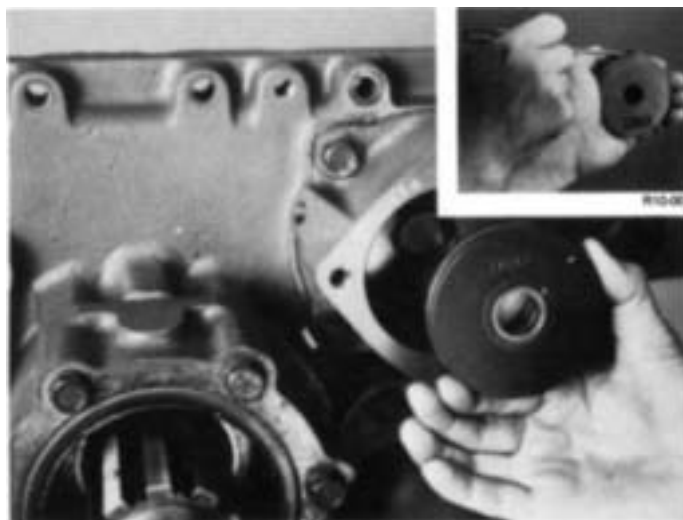
6. Remove the range piston from cylinder bore. If necessary, remove the O-rings from piston I.D. and O.D. (inset).
