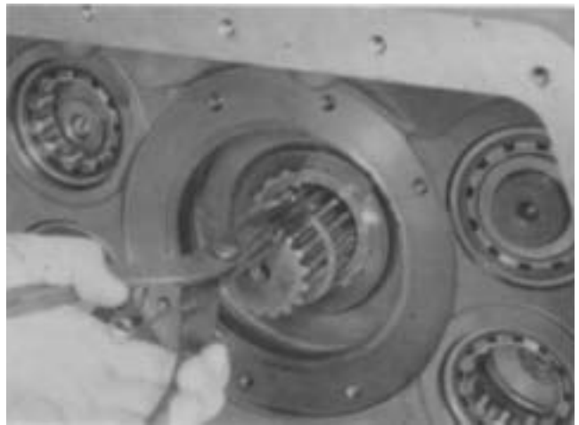
7. Remove the inner snap ring from the mainshaft.
