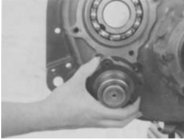
3. Remove the reduction cylinder body and yoke bar.
