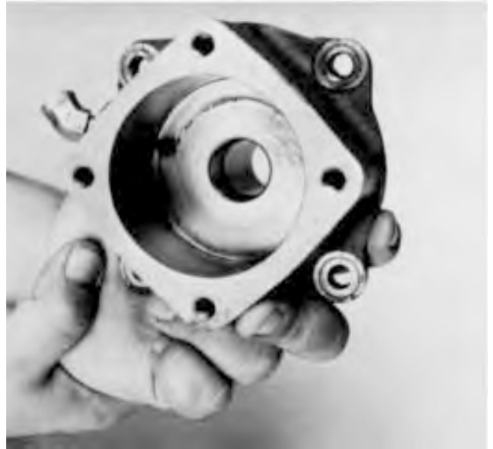
8. If necessary, remove the small O-ring from the range cylinder housing bore.
