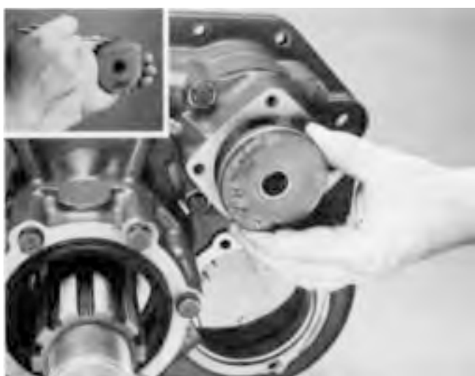
6. Remove the range piston from the cylinder bore. If necessary, remove the O-rings from the position I.D. and O.D. (inset).
