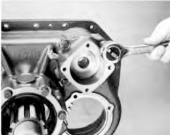
7. Remove capscrews and range cylinder housing.
