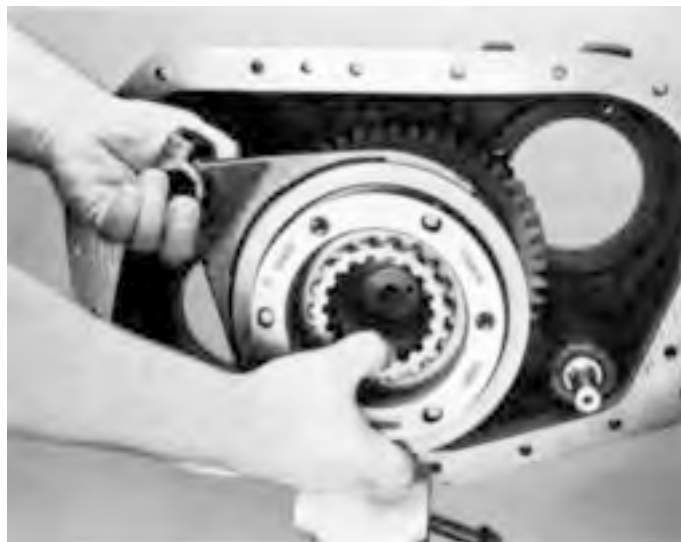
5. Remove the shift yoke and synchronizer assembly from output shaft.
