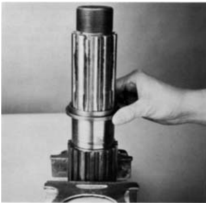
6. Remove the stepped washer from shaft of models so equipped.
