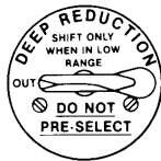
Lever to "IN" (Valve CLOSED)
