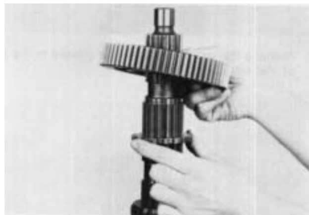
17. Remove 1st speed gear and splined washer from mainshaft.
