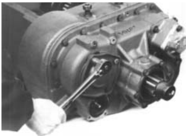
5. Install the rear bearing covers.
