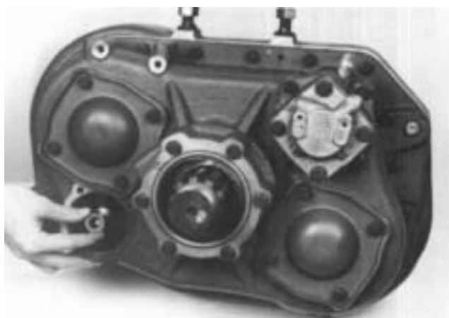
6. Install the gasket on the intermediate shift shaft.
