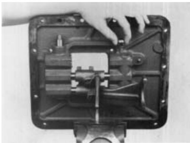
5. Install an interlock ball in the front web.
