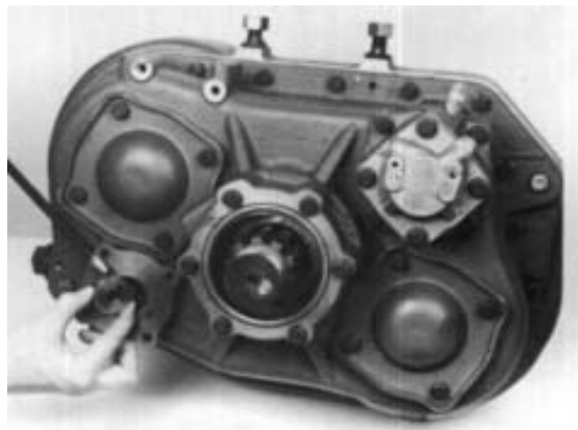
8. Install the O-ring on the outer diameter of the piston and install the piston on the shaft in the cylinder. Lubricate O-ring with silicone.
