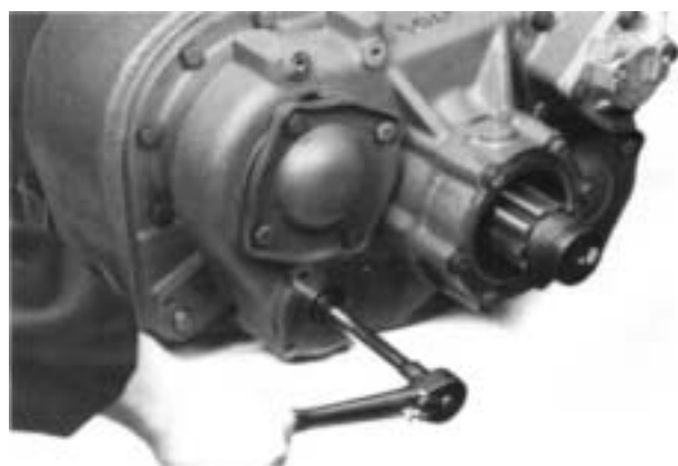
9. Install the elastic stop nut on the shaft.
