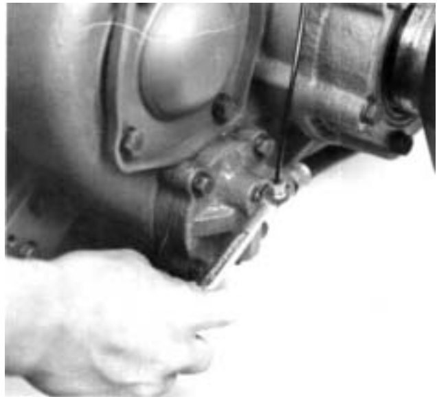
7. Disconnect the black 1/8" O.D. signal line at the intermediate cylinder.
