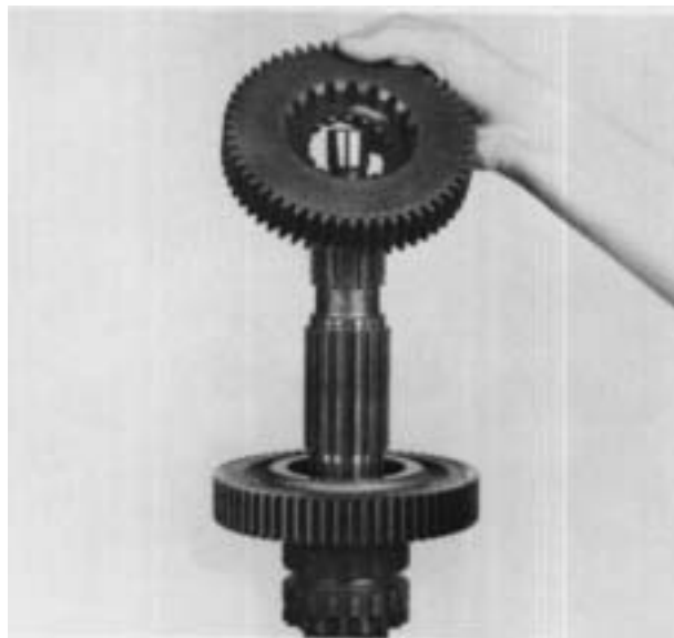
16. Remove 2nd gear and splined washer from mainshaft.
