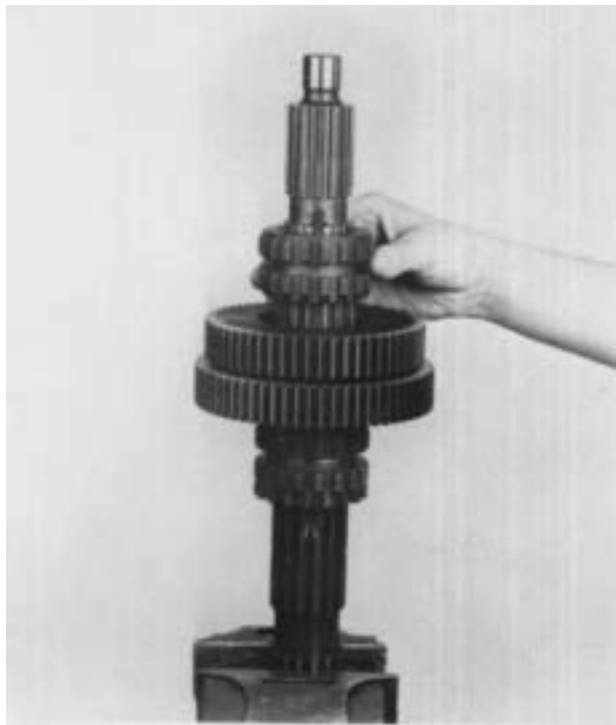
14. Remove the 2nd-3rd speed sliding clutch.
