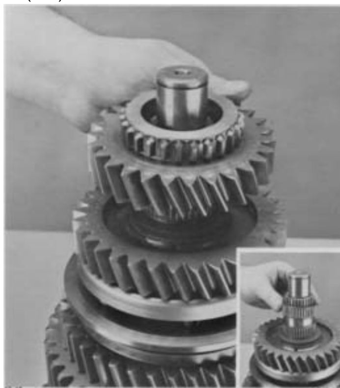
17. Install locating ball and washer. Washer can be installed either way. Install snap ring as shown (inset).
