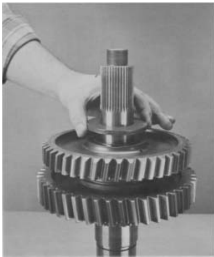
8. Install reverse gear washer. Washer can be installed either way.
