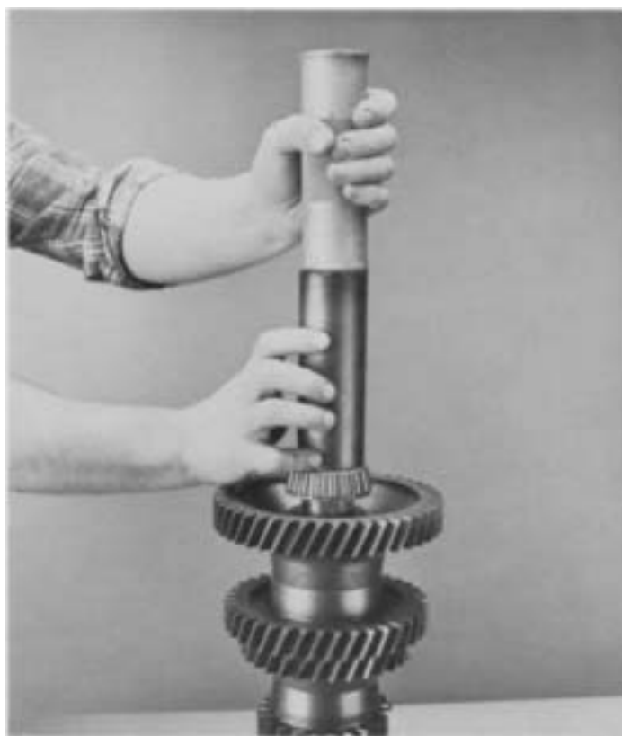
6. Install front countershaft bearing as shown.
