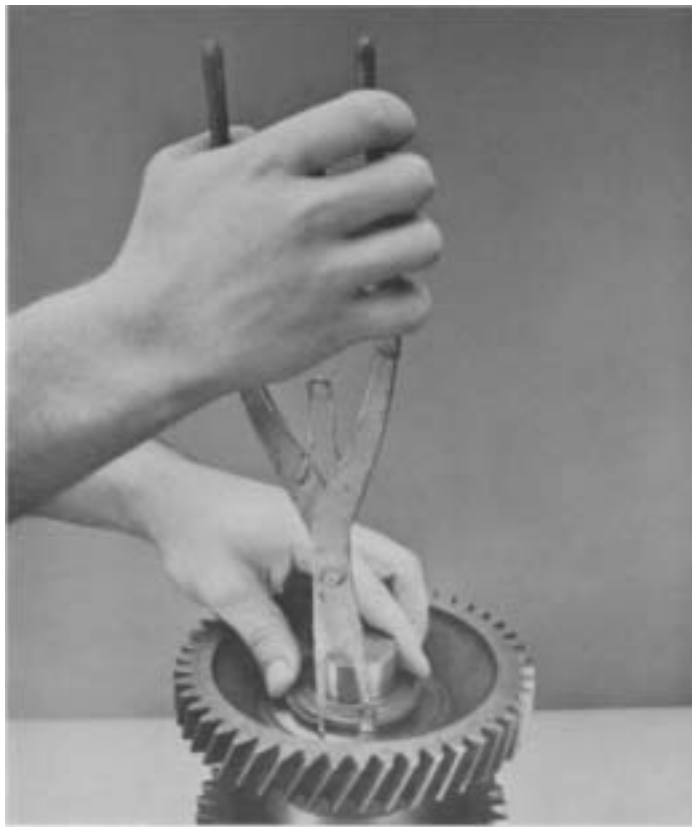
5. Install snap ring in groove at front of countershaft.
