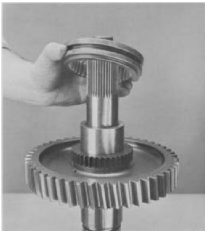
5. Install reverse gear sliding clutch with stepped shoulder down.
