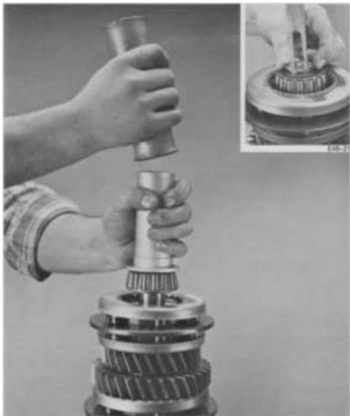
21. Using a sleeve type driver install front mainshaft bearing. Install snap ring in groove on end of shaft (inset).
