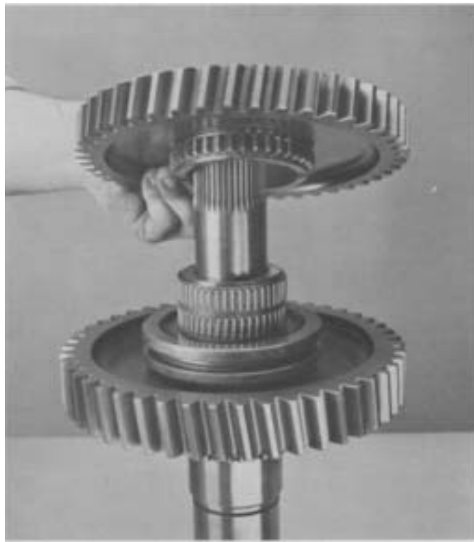
7. Install reverse gear with clutching teeth facing down.
