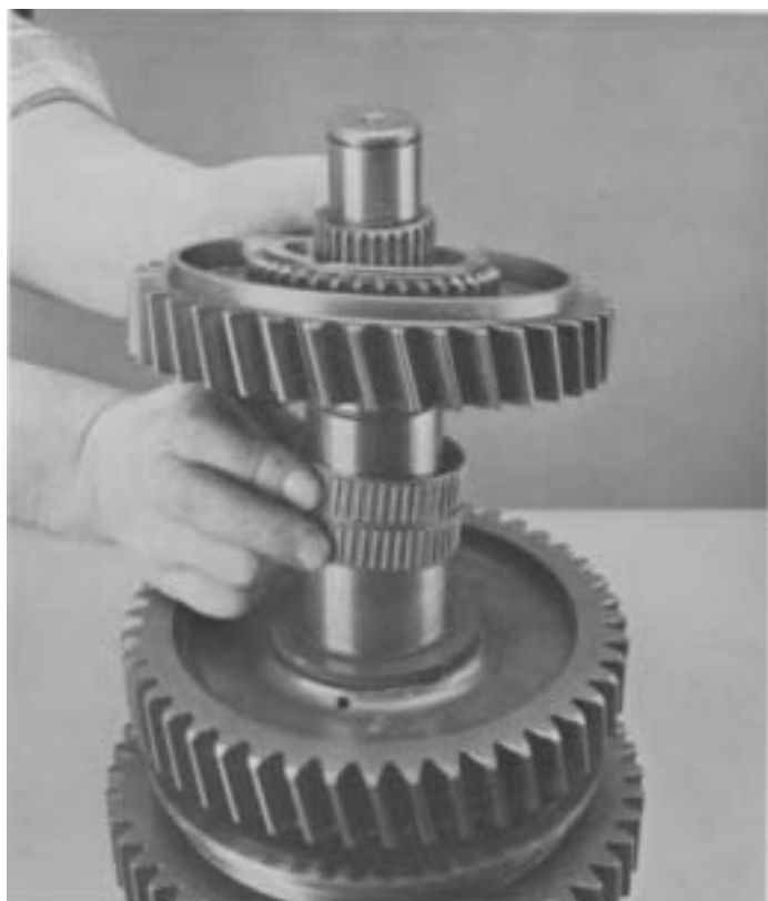
11. Remove 3rd gear and bearings from mainshaft.
