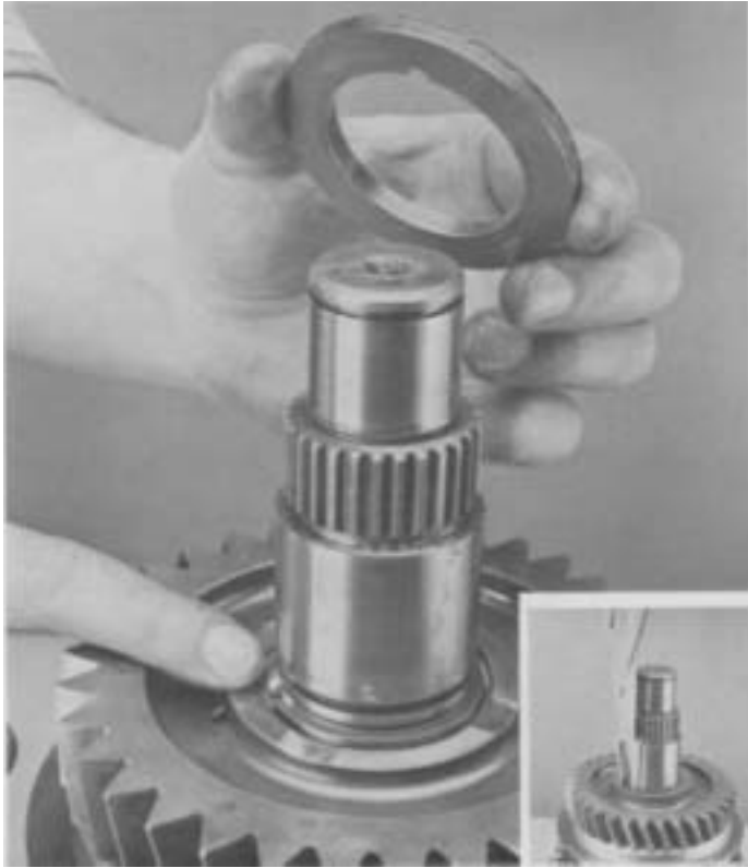
7. Remove snap ring (inset), thrust washer, and locating ball.
