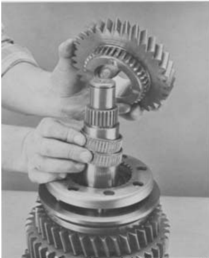
8. Remove 4th gear and bearings
