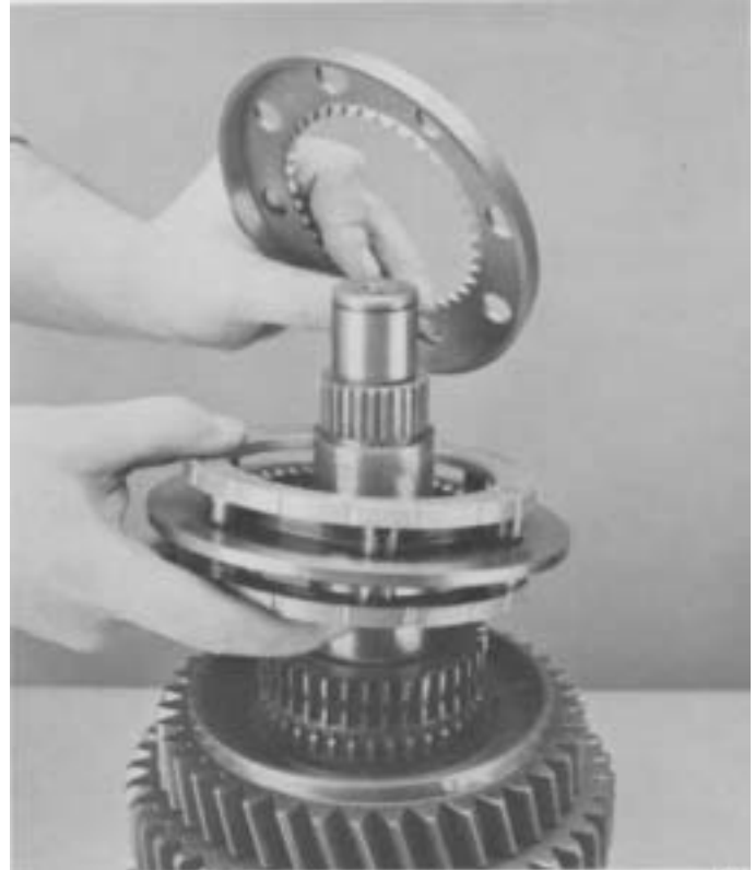
9. Remove 4th speed synchronizer cup and 3rd-4th speed synchronizer
