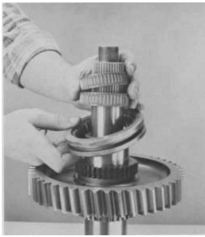
17. Remove reverse gear bearings and reverse gear
