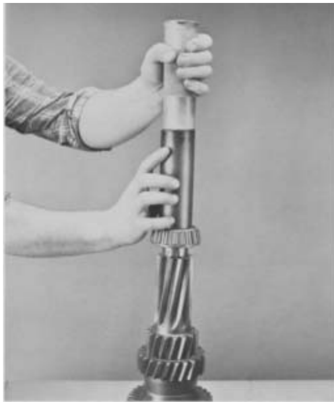
7. Install rear countershaft bearing as shown.
