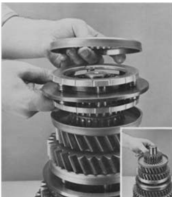
20. Install 5th speed synchronizer cup (inset). Lubricate friction surface with transmission lube and install 5th-6th speed synchronizer assembly and 6th speed synchronizer cup.
