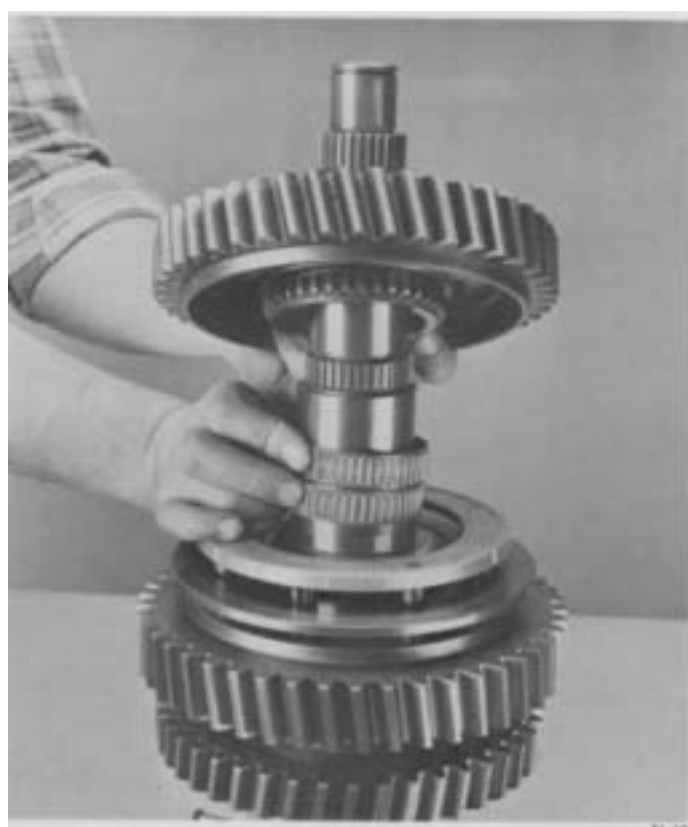
11. Remove 3rd gear and bearings from mainshaft.
