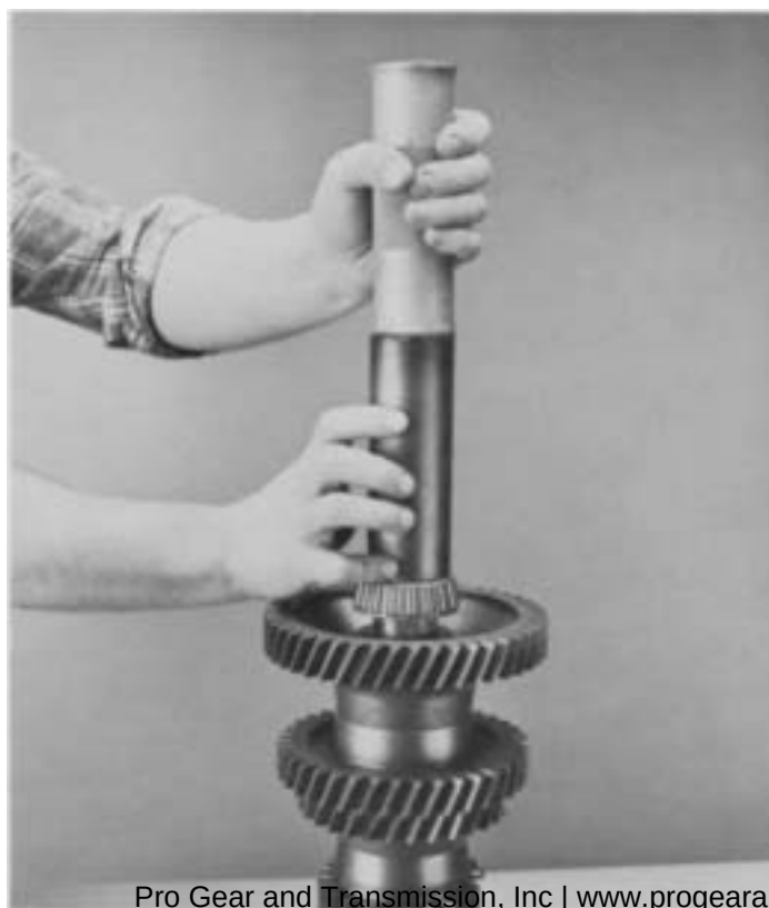
6. Install front countershaft bearing as shown.
