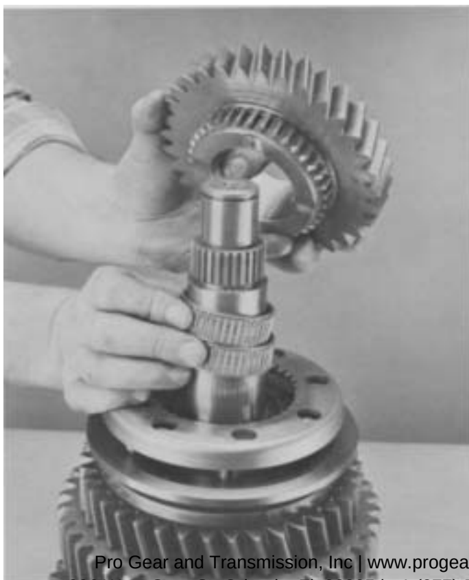
7. Remove snap ring (inset), thrust washer, and locating ball.
