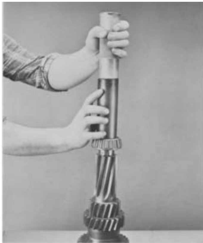
7. Install rear countershaft bearing as shown.
