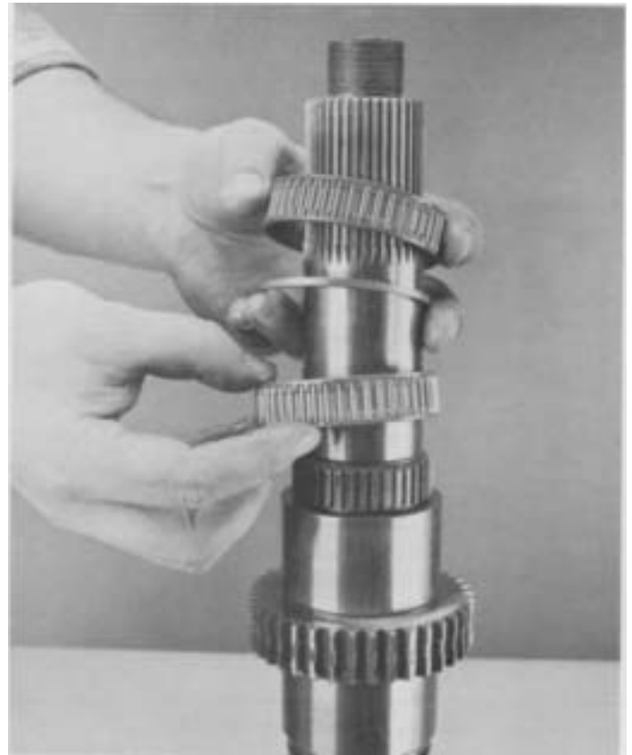
19. Remove first gear bearing and spacer.
