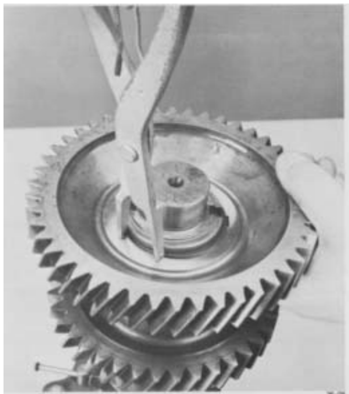
9. Remove drive gear retaining snap ring from front of shaft.
