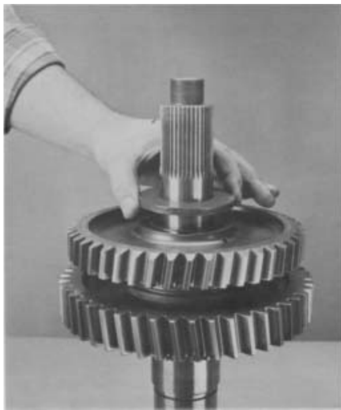
6. Lubricate and install reverse gear bearings on race. 906 West Gore St, Orlando, FL 32805 | +1 (877)-776-4600 | +1 (407)-872-191 | parts@eprogear.com 8. Install reverse gear washer. Washer can be installed either way.
