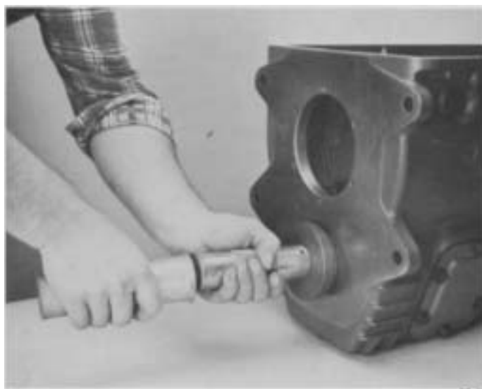
8. If previously removed, install snap ring, countershaft front bearing race (from inside of case) and bore plug. Coat outer diameter of bore plug with Loctite #510 before installing.
