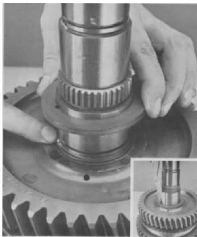
12. Remove snap ring (inset), thrust washer and locating ball.
