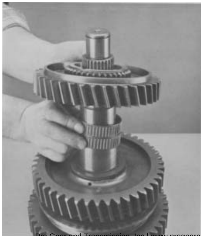
11. Remove 1st gear and bearings from mainshaft.
