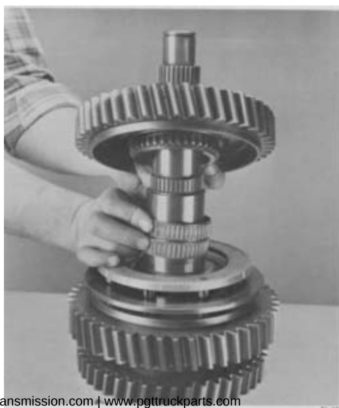
13. Remove 2nd gear and bearings from mainshaft.
