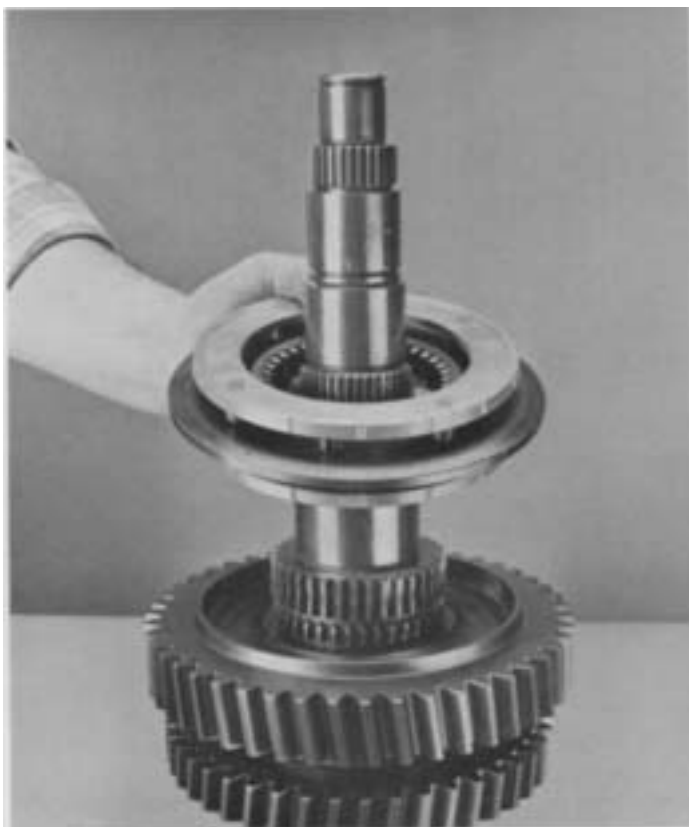
14. Remove 1st-2nd speed synchronizer.
