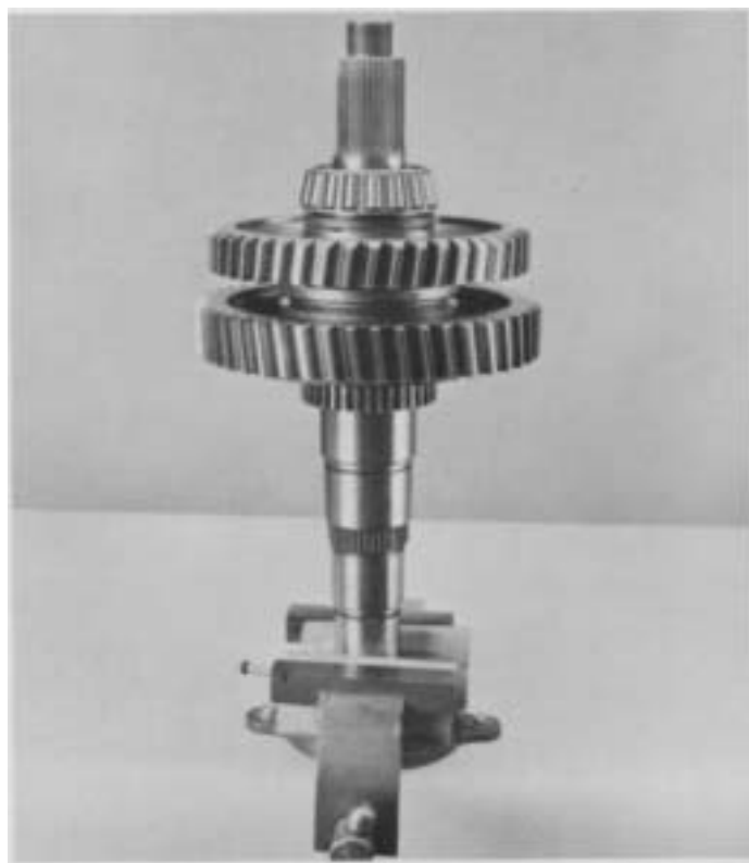
15. Reposition mainshaft in vise, rear of shaft facing up.
