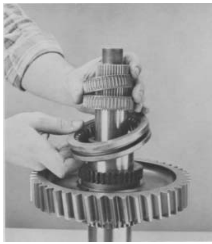
15. Reposition mainshaft in vise, rear of shaft facing up.
