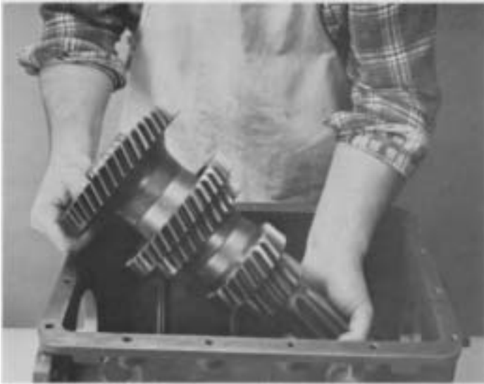
9. Carefully lower countershaft into case.
