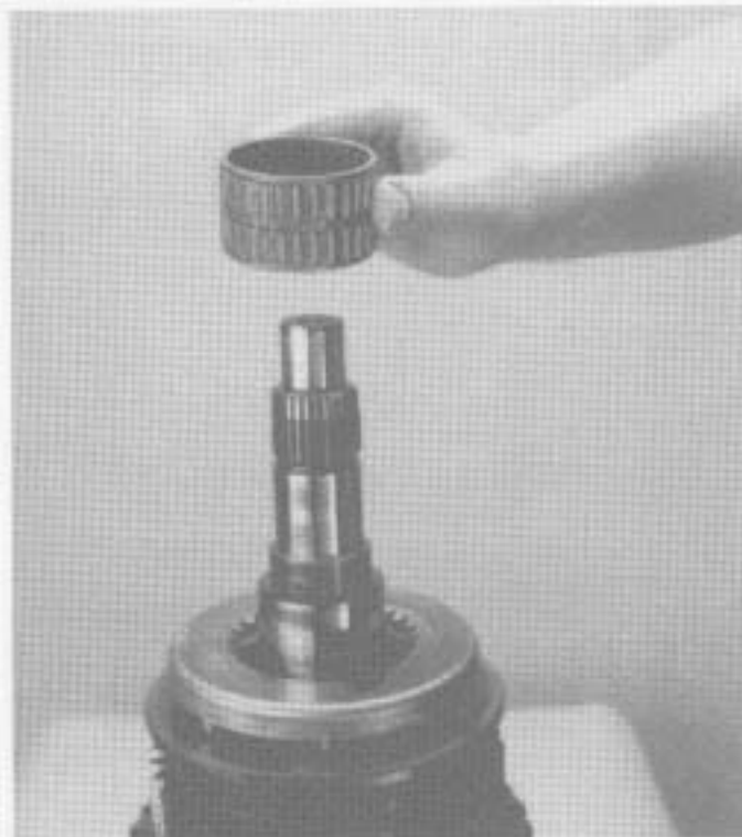
17. Install mainshaft 3rd speed gear bearing.
