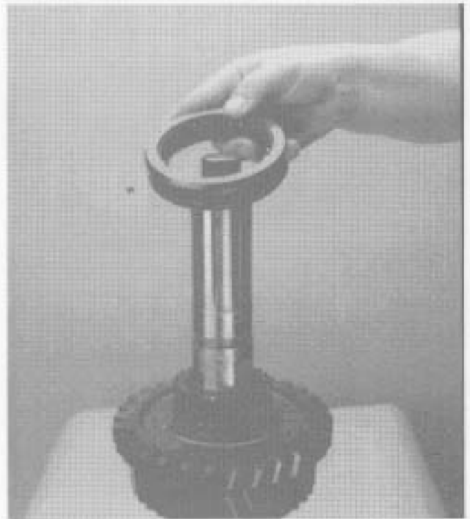
8. Install 1st-reverse gear sliding clutch.
