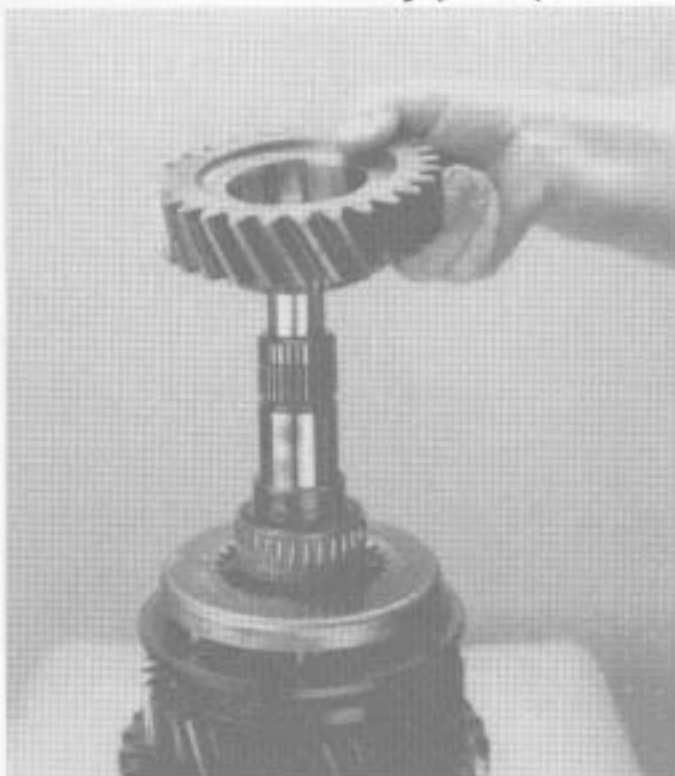
11. Remove the 3rd speed gear.
