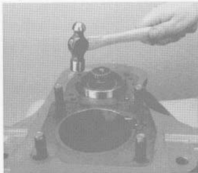
11. Install the countershaft rear bearing race into the transmission case as shown.
