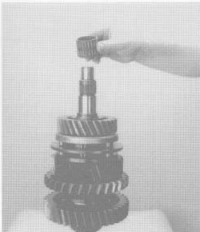
21. Install mainshaft 4th gear bearing.
