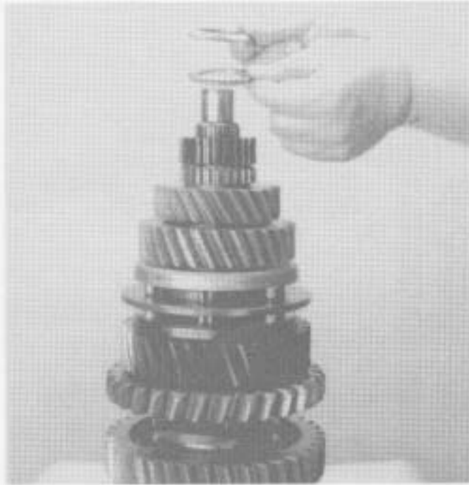
24. Install thrust bearing and bearing race on the mainshaft 4th-5th clutch hub.
