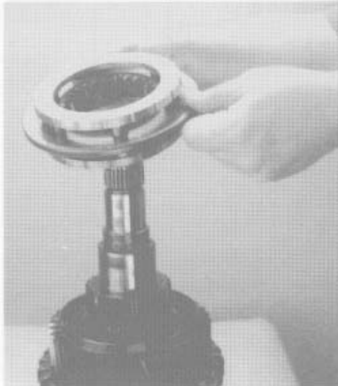
15. Reposition mainshaft in vise so front is up. Install the mainshaft 3rd speed gear synchronizer assembly.
