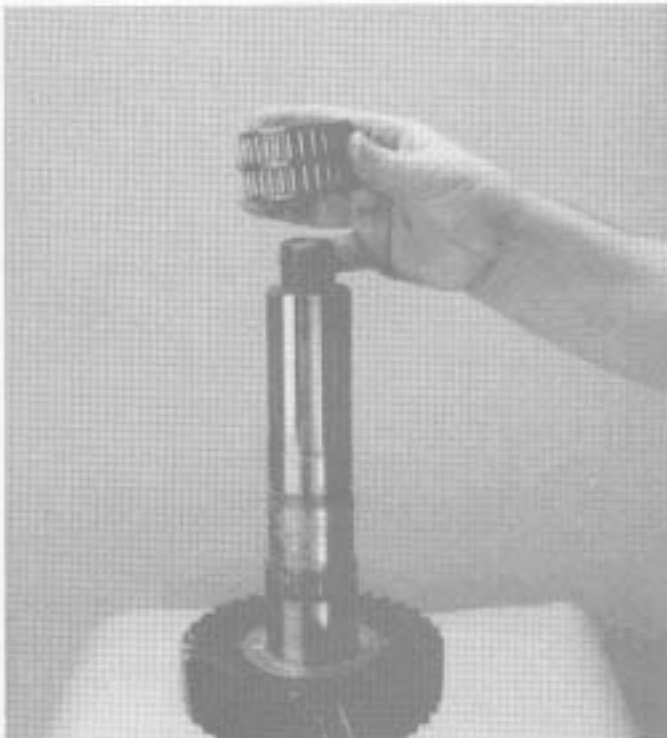
24. Remove the reverse gear bearing.
