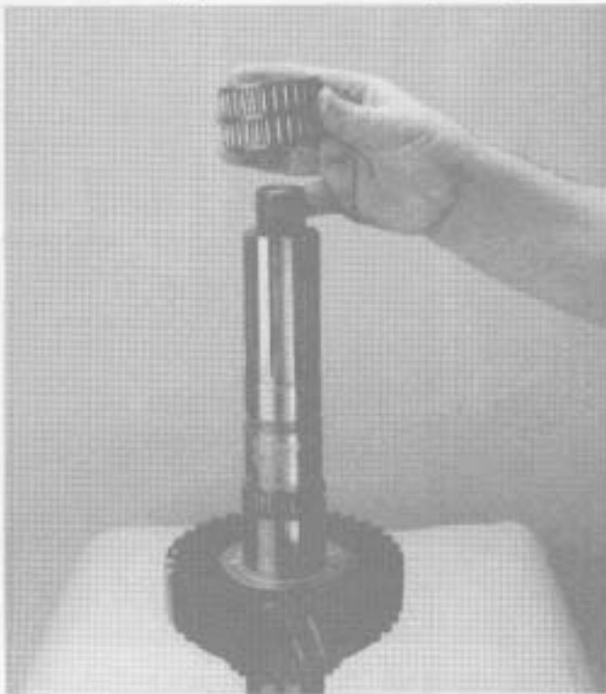
5. Install mainshaft reverse gear bearing.
