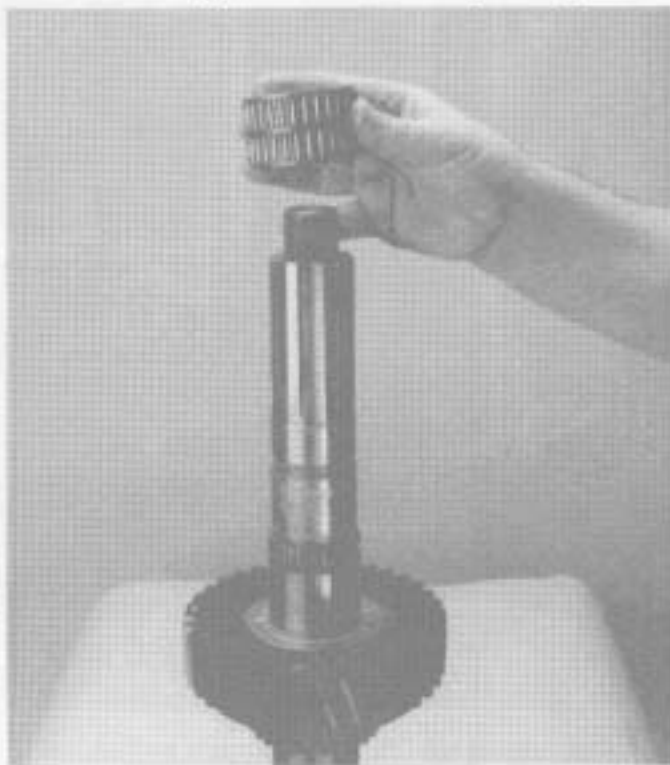
5. Install mainshaft reverse gear bearing.
