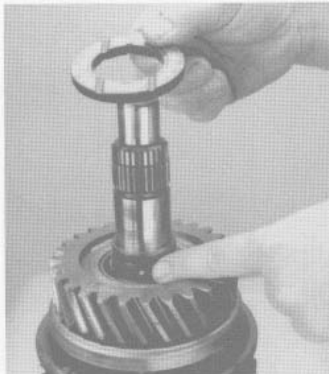
19. Install locating ball and 3rd speed gear thrust washer.
