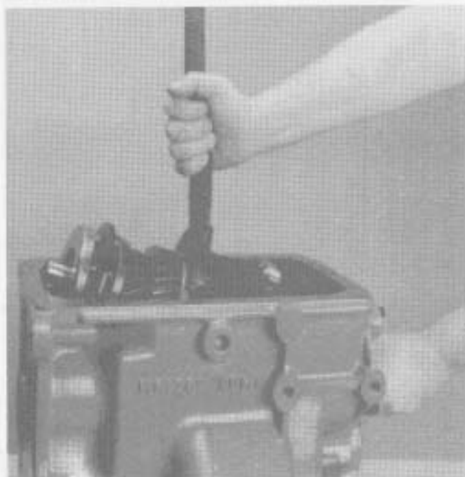
26. Remove the mainshaft from the vice and wrap a sling or rope around 2nd-3rd synchronizer. Use a hoist to install the mainshaft assembly in transmission case.
