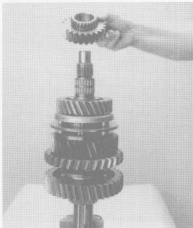
7. Remove the 4th speed gear.
