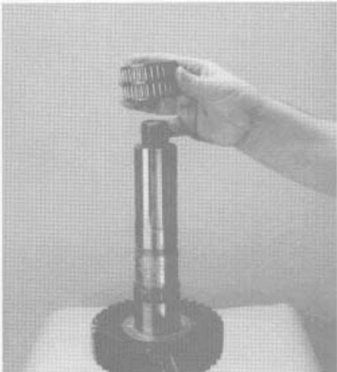
24. Remove the reverse gear bearing.
