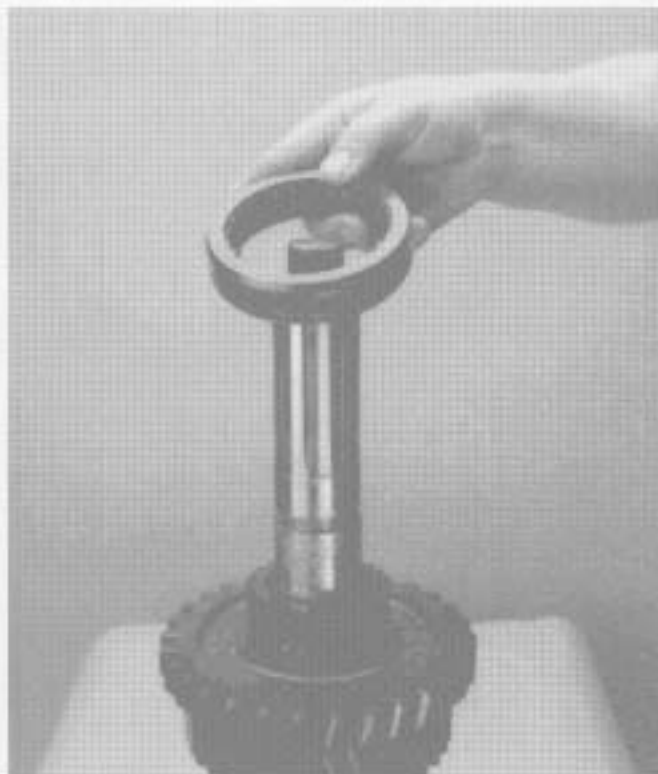
21. Remove the 1st-reverse sliding clutch.
