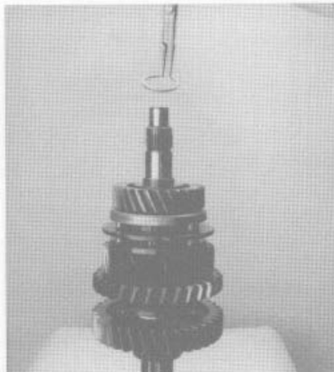
20. Install mainshaft 3rd speed gear retaining snap ring in the snap ring groove.
