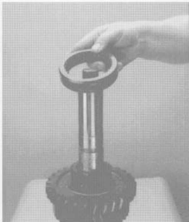
21. Remove the 1st-reverse sliding clutch.
