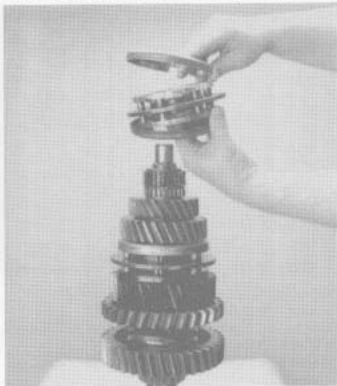
25. Install 4th-5th speed synchronizer and cups over the mainshaft 4th-5th clutch hub.
