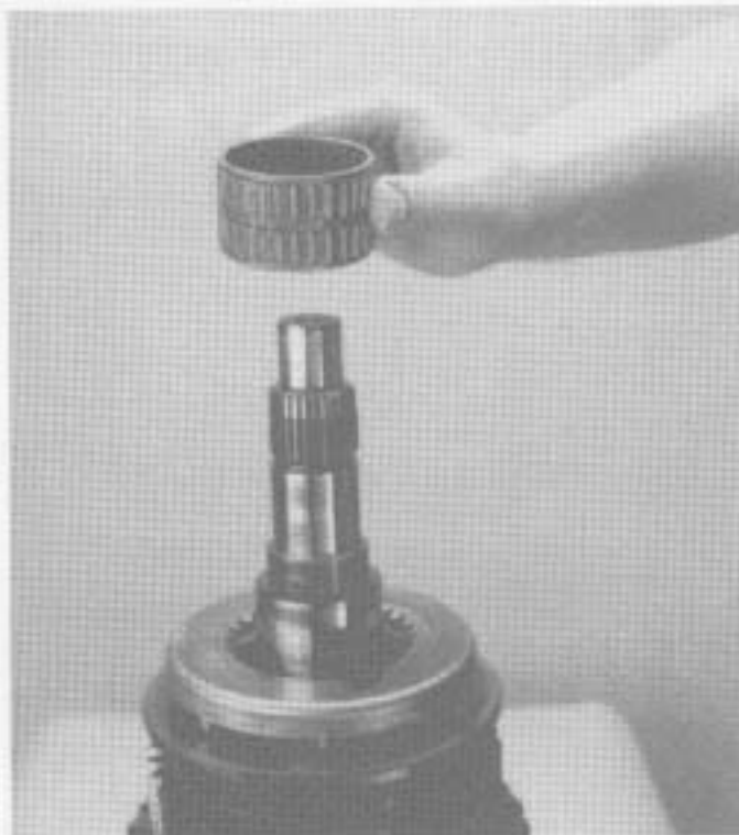
17. Install mainshaft 3rd speed gear bearing.
