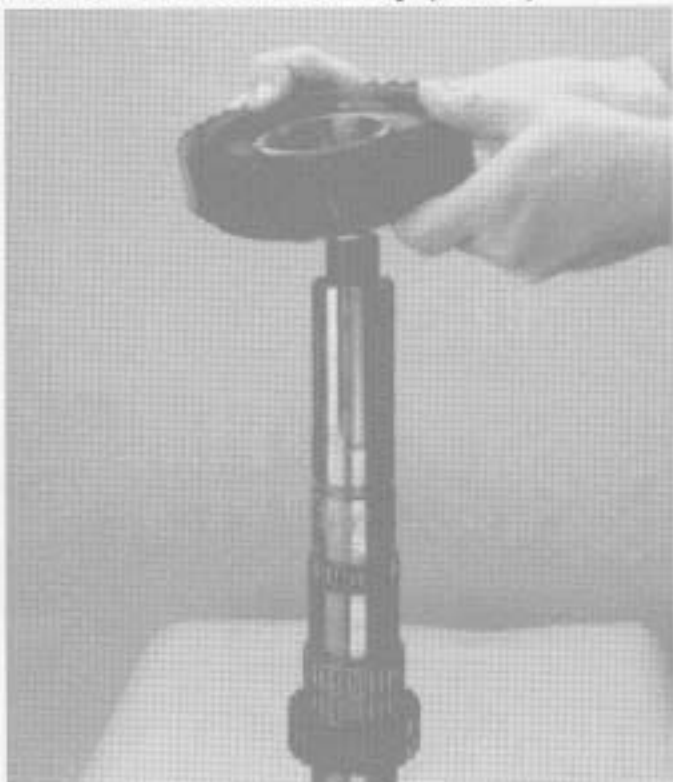
27. Remove 2nd speed gear.
