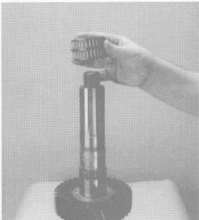
24. Remove the reverse gear bearing.
