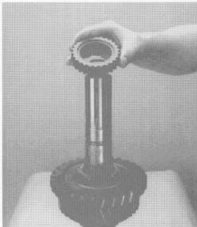
7. Install mainshaft 1st-reverse speed clutch hub.
