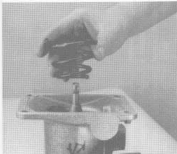
3. Remove the tension spring from the housing.
