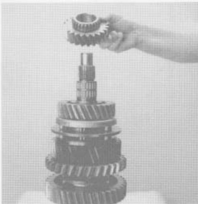
22. Install mainshaft 4th speed gear, clutching teeth facing up.
