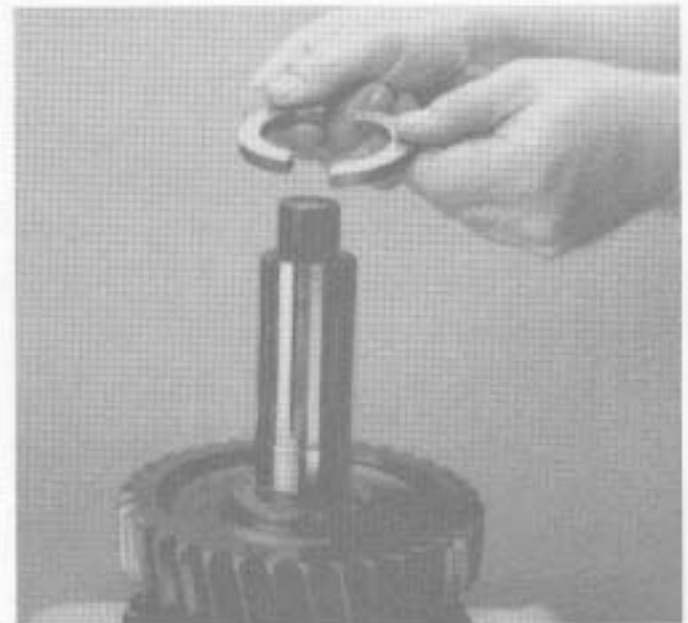
12. Install a locating ball on the mainshaft. Install 1st speed gear split washer, so the split rings join at the locating ball.
