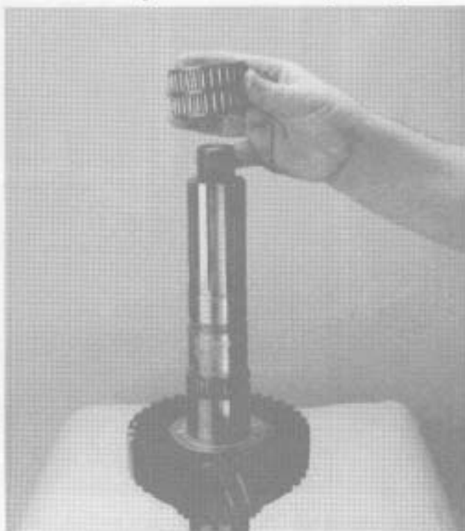
5. Install mainshaft reverse gear bearing.
