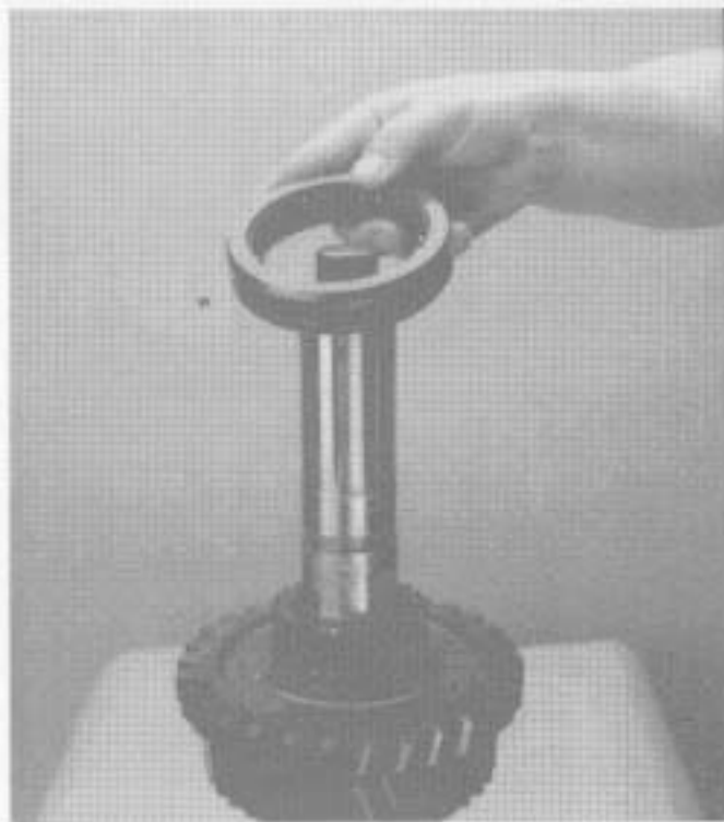
8. Install 1st-reverse gear sliding clutch.
