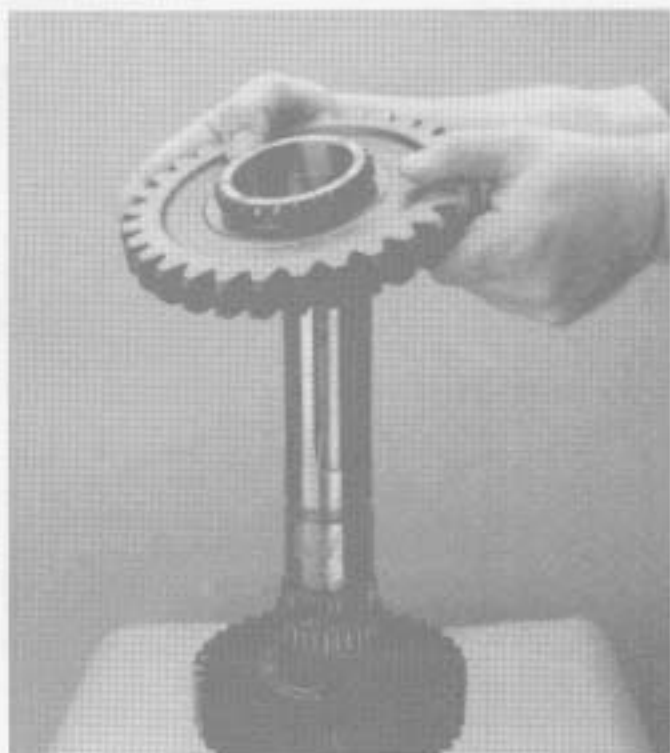
6. Install mainshaft reverse gear.
