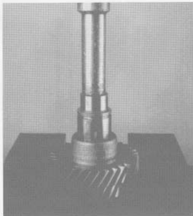
12. Remove countershaft 4th gear.
