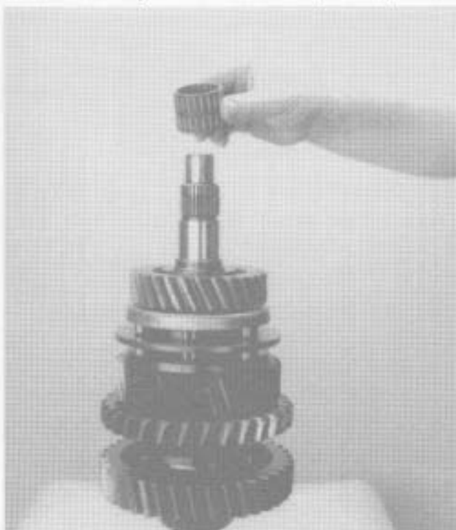
21. Install mainshaft 4th gear bearing.
