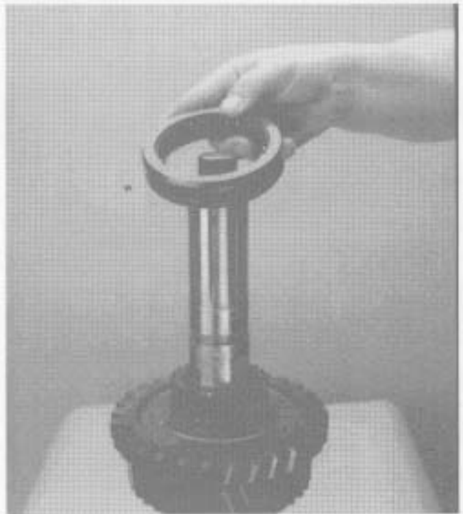
8. Install 1st-reverse gear sliding clutch.
