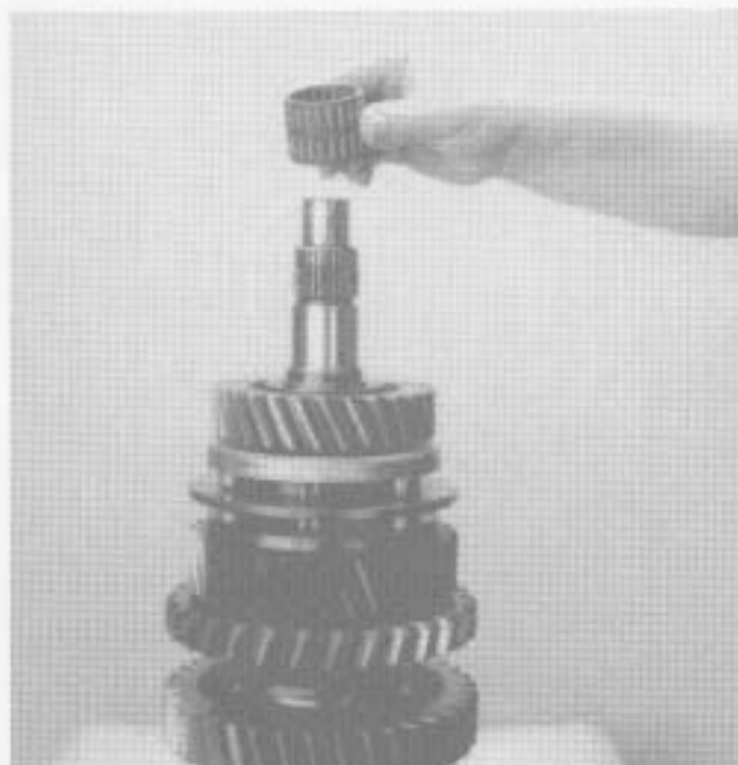
8. Remove 4th gear bearing.
