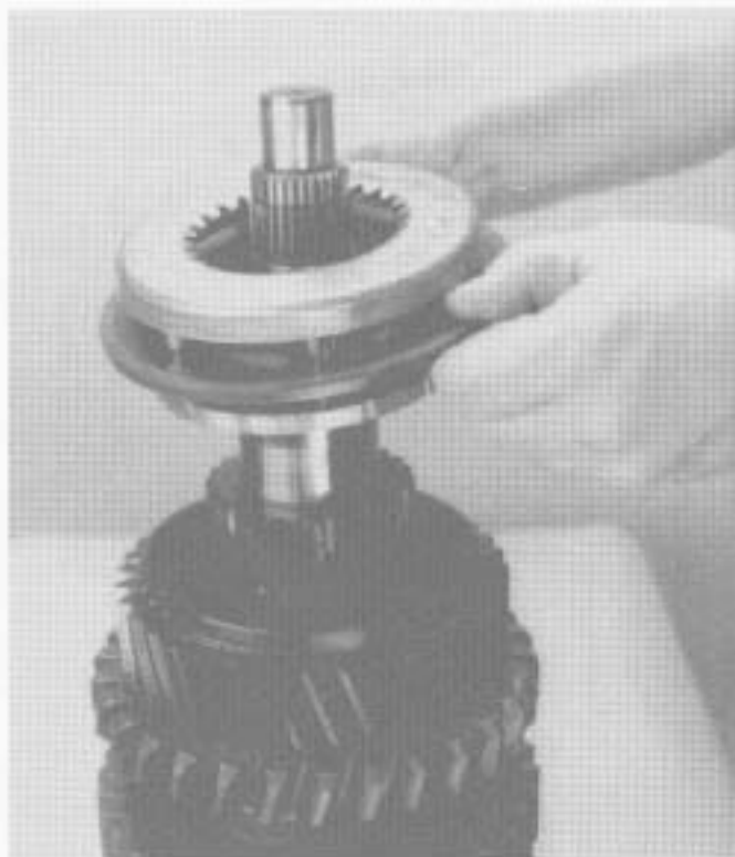
13. Remove the 3rd gear synchronizer cup and synchronizer assembly.
