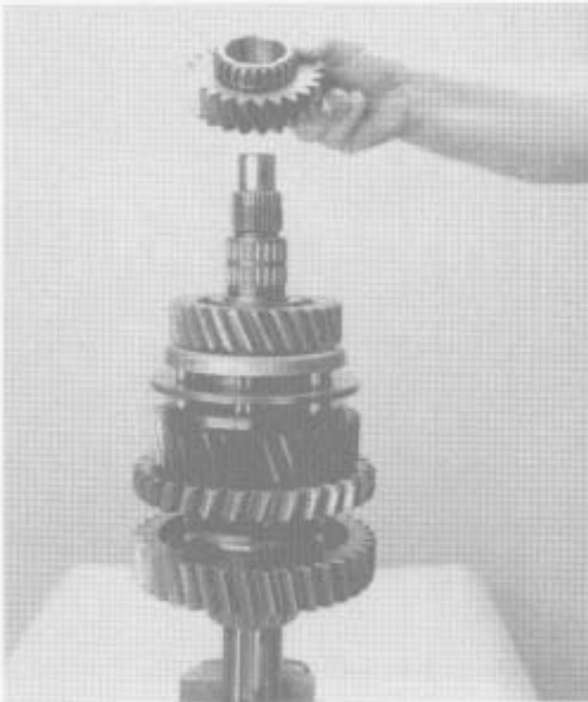
7. Remove the 4th speed gear.
