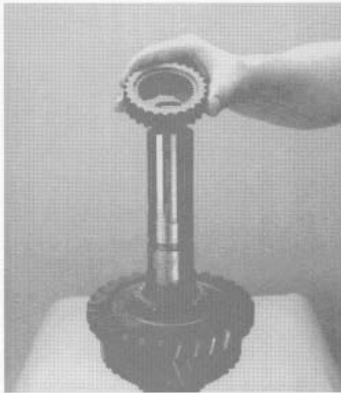
7. Install mainshaft 1st-reverse speed clutch hub.
