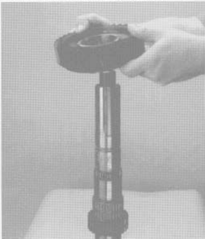
27. Remove 2nd speed gear.
