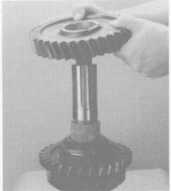
11. Install mainshaft 1st gear over the two rows of needle bearings, with clutching teeth down. Be careful not to catch the needle roller bearings.
