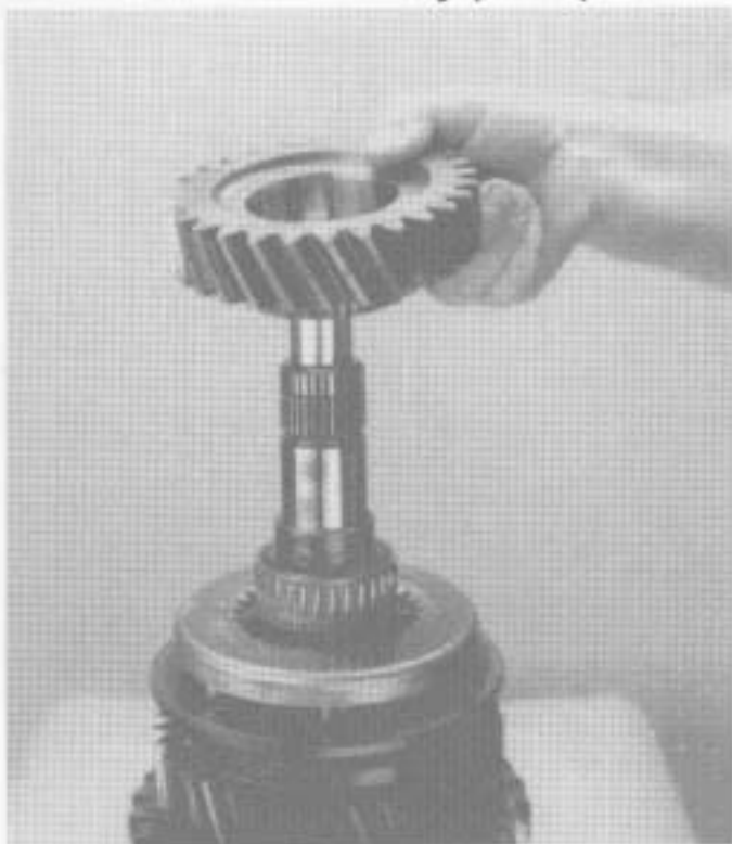
11. Remove the 3rd speed gear.
