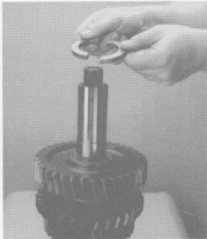
17. Remove the 1st gear split washer.
