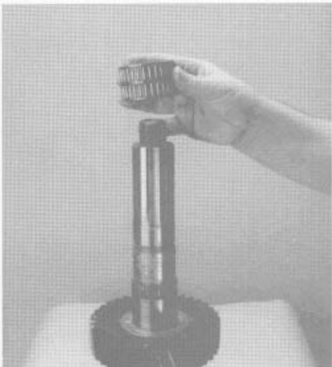
24. Remove the reverse gear bearing.
