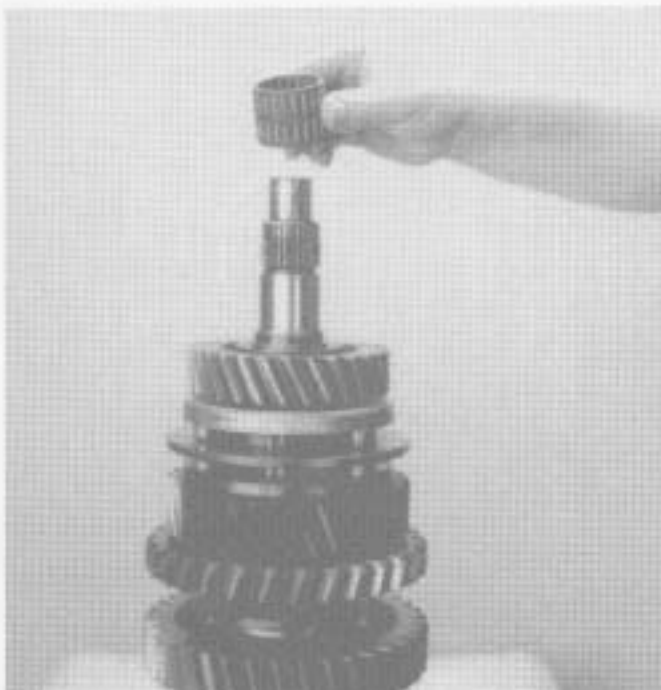
8. Remove 4th gear bearing.
