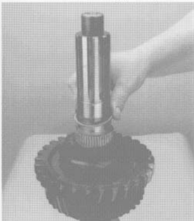
19. Remove the bearing rollers and spacers.
