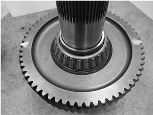
Two Marked Teeth 180 Degrees Apart
